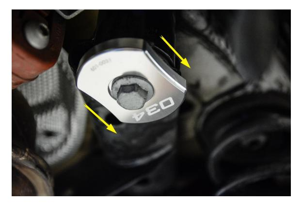
**Step 8** – Using an 18mm Socket, remove the front bolt securing the rear subframe to the chassis.
