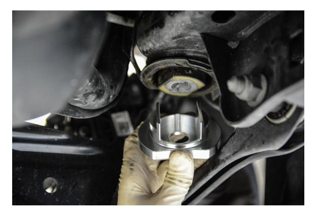
**Step 11** – Install rear subframe insert by pressing into the rubber voids of the factory rubber subframe bushing. We recommend aligning the insert such that the 034 logo is toward the front of the car.
