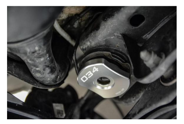
**Step 12** – Install subframe bolt using an 18mm Socket. **Note:** We recommend replacing the original subframe bolts with new pieces, as they are stretch bolts that are intended for a one-time use. **If you opt to reuse the stock bolts, torque them to 90 Nm with Blue Loctite.**
