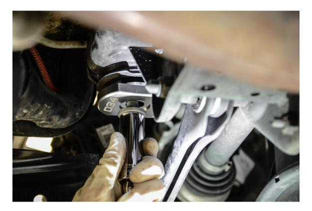
**Step 13** – Torque subframe bolt to 70 Nm + 180° Turn. (Arrows point toward the front of the car for reference)
