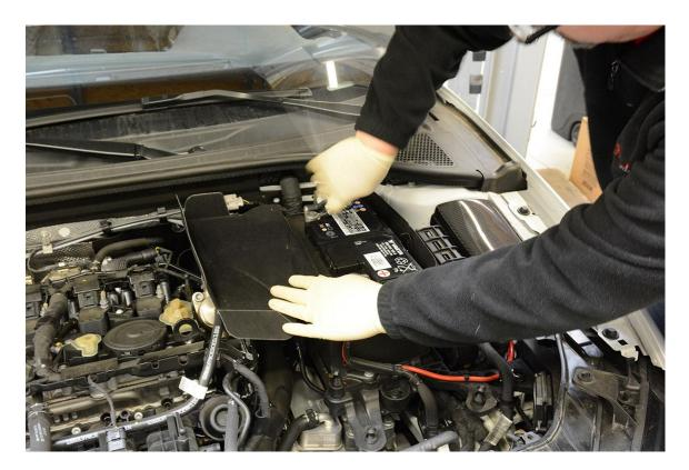
**Step 9** – Remove the battery holder bracket after loosening the bolt with a 13mm socket. Remove the battery blanket, and carefully lift the (heavy) battery out of the engine bay. Do a few reps if you're looking for gains.
