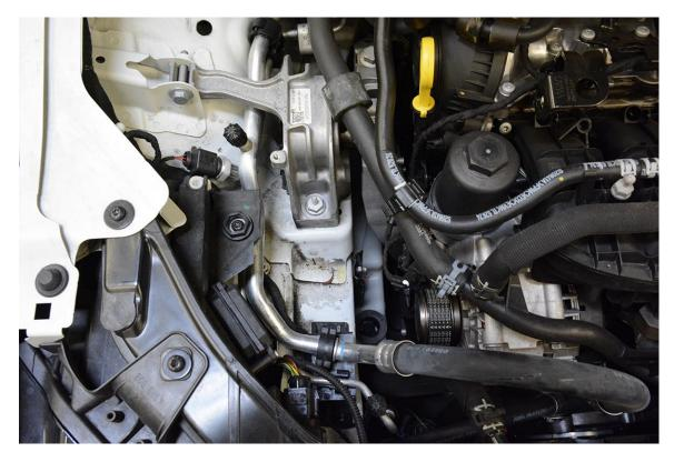
**Step 20** – Use an engine support to support the engine/transmission assembly via the factory lift points.
