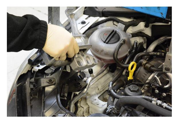
**Step 29** – the new Street Density Engine Mount. Secure using the bolt to the body, two bolts to the frame rail, and two bolts to the engine.
