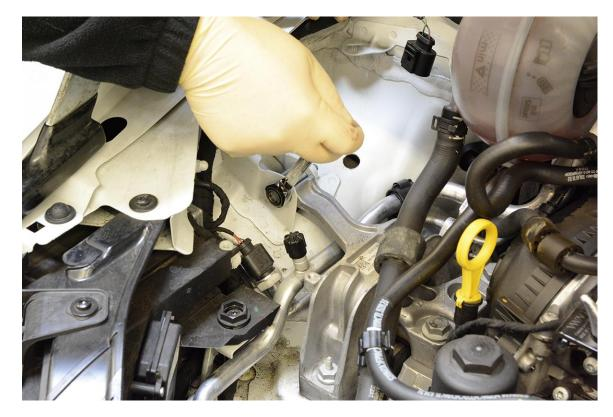
**Step 22** – Using a 16mm socket, remove the two bolts securing the Engine Mount to the frame rail.
