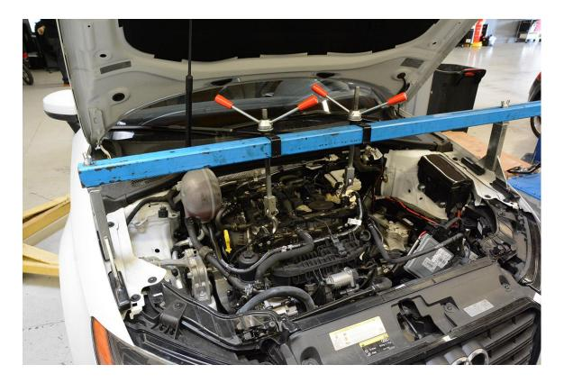
**Step 21** – Using a 13mm wrench, remove the bolt securing the Engine Mount to the body.
