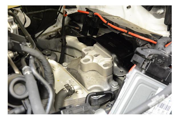
**Step 27** – Using an 18mm socket, remove the 2 bolts securing the Engine Mount to the engine.
