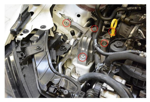
**Step 30** – Secure the Transmission Mount to the transmission with three factory bolts.
