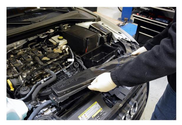
**Step 7** – Remove the factory lower airbox by lifting up firmly.
