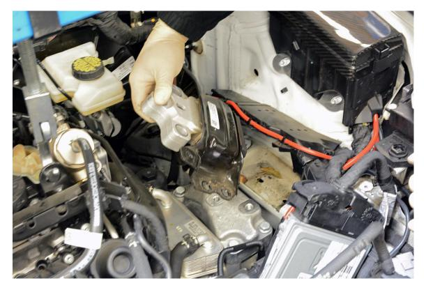
**Step 26** – Install the new Street Density Transmission Mount, and secure to the frame rail using four factory bolts.
