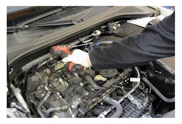
**Step 4** – Remove the 8 T25 Torx screws securing the upper airbox. Remove the breather hose from the front left side of the factory airbox. If your vehicle is equipped with SAI, remove the secondary air injection hose from the upper airbox. Now, remove the airbox and intake tube from the engine bay.
