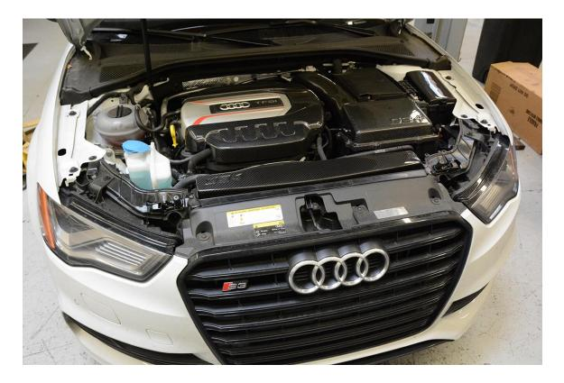
**Step 2** – Remove the engine cover by pulling up firmly.
