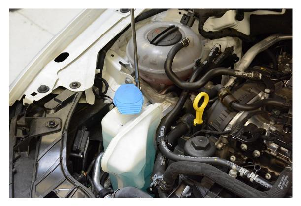
**Step 16** – Unplug the connector to the coolant level sensor.
