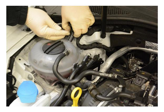
**Step 17** – Lift the coolant reservoir up and tuck out of the way to allow for access to the Engine Mount.
