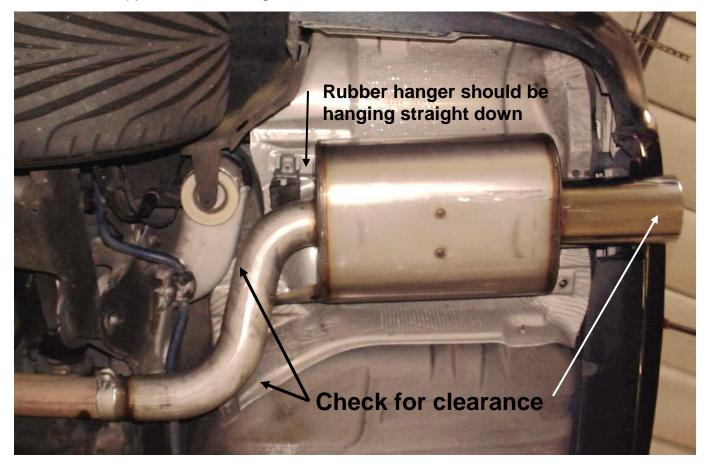
8. Visually inspect the muffler. Check for  $\frac{1}{2}$  clearance in all areas. Make sure the polished tip is centered in the opening and has at least a finger's clearance from the body.
