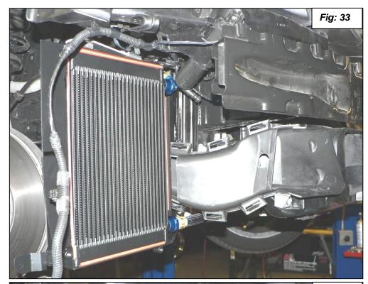
43. When you pull the cooler into the position it will be with the bumper attached, and the clearance should be flush. See figure 34.
