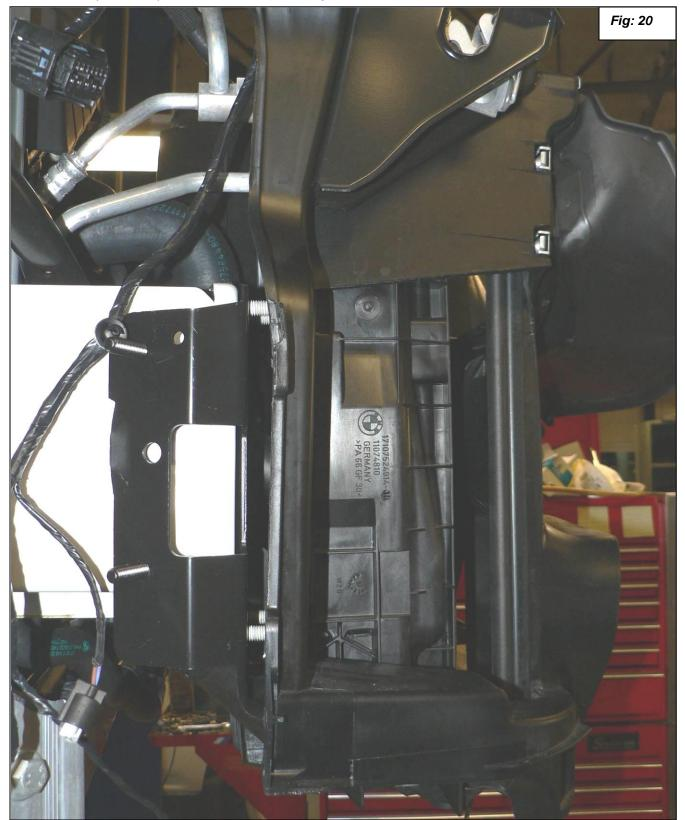
29. Cut off part of the plastic mount that is not needed. You will need the space for clearance for the oil cooler. See figures 21 and 22.
