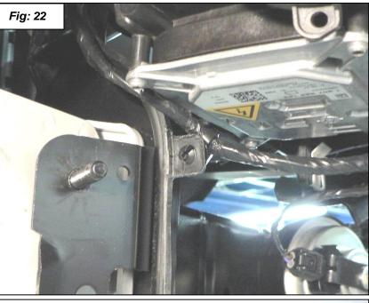
31. Install the top support bracket onto the new Dinan oil cooler mount with the supplied 6mm x 10mm bolts and washers. Install the rubber mounts. See figure 23.
