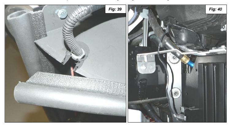
**48**. Install the bumper over the air duct after connecting the fog light on the passenger side as you install it.
