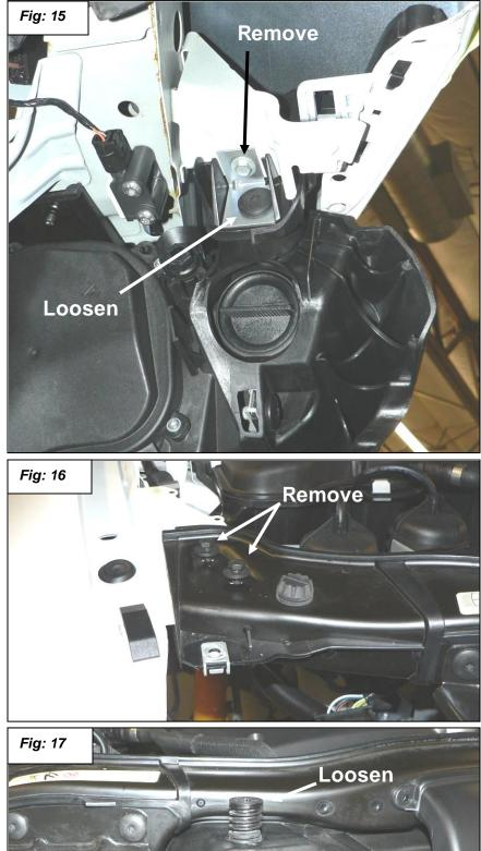
24. Remove the two 10mm hex head bolts from both sides of the upper radiator support as shown in figure 16.
