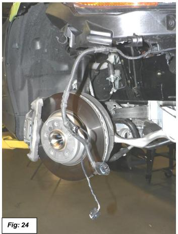
33. Remove the tape and plastic tube that covers the wires as shown in figure 25.
