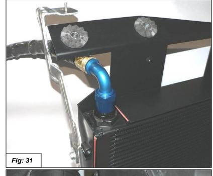
38. Feed the oil line in between the headlight and the bracket as shown in figure 32. Attach the oil cooler assembly to the mounts as shown with the two stock 8mm nuts and the 6mm bolt. Torque nuts to 20Nm (15ft-lbs.) and bolt to 8Nm (6ft-lbs.). See figure 32.
