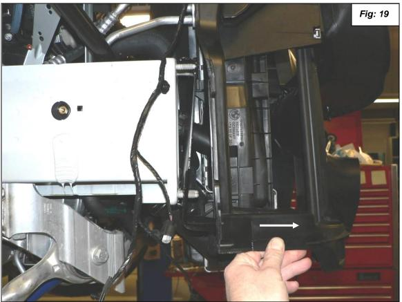
28. Slide the supplied new BMW part number 51 64 7 154 546 lower radiator support bracket with mount for oil cooler onto the studs where the other one without the mount for oil cooler was. See figure 20. Install nuts, bolts, screws and radiator mount in reverse order of removal. Torque bumper nuts to 22Nm (16 ft-lbs.). You do not need to replace rivets.
