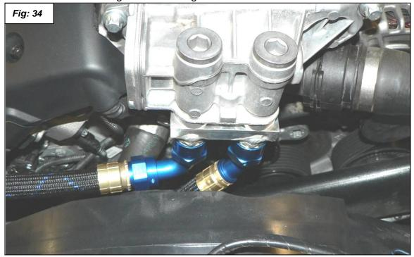
41. Check line for best routing and tighten fittings with 2 wrenches, one on hose fitting and the other on fitting attached to oil cooler or adapter block.
