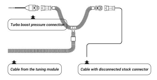
• Disconnect the plug from turbo boost pressure sensor.
