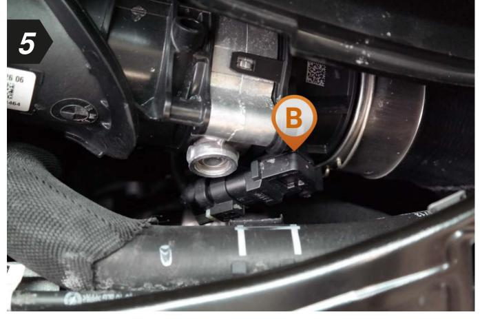
• To begin, locate the turbo boost pressure sensor in your engine bay.
