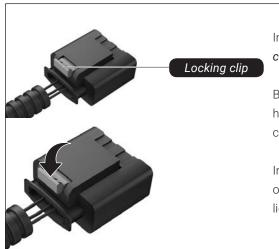
In the first step, the grey *locking clip* is pulled out. Press the grey *locking clip*, which functions as a lever for loosening the plug and pulling it out.
