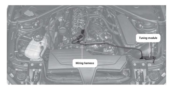
• Before fixing the tuning module in place in the engine bay, ensure that the wiring harness can also be routed and fixed securely without putting it under excessive tension.
