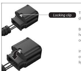
The plugs are locked into the connection sockets by means of a locking clip. Press the *locking clip* and pull the plug.
