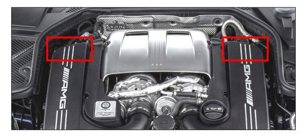
3. Release the 4 clamps indicated below, and remove both airbox assemblies from the car by pulling upwards. Also release the locking tabs and remove both intake ducts from the car.
