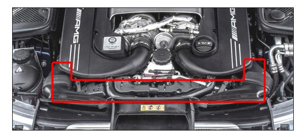
Work your way around the assembly and remove the bolts securing the harness assembly to the engine.
