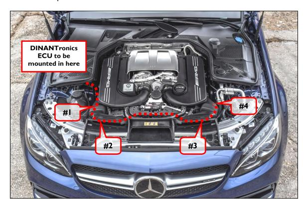
2. Remove the two covers indicated below, and unplug the ambient temperature sensors (one on each side). Do not remove the sensors.
