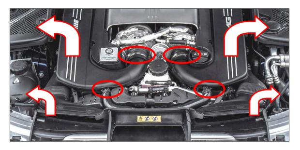
4. The sensors are located underneath an engine wiring harness, which is secured to a series of plastic covers above it, and this assembly is attached to the engine with a number of bolts and plastic barbed fasteners. This assembly must be released from the engine and allowed to slide forward about 5"-6", in order to provide access to the sensors underneath.
