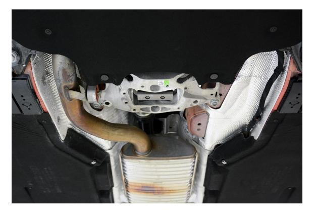
**Step 2** – Using a 10mm Triple Square, remove the two M8 bolts securing the factory transmission mount bracket to the transmission mount assembly.
