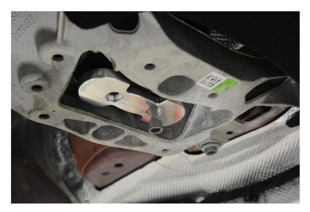
**Step 5** – Torque the factory M8 bolts to 25 Nm with Blue Loctite applied. Make sure to thread in both bolts before tightening either of them to spec to ensure that the insert is properly lined up.
