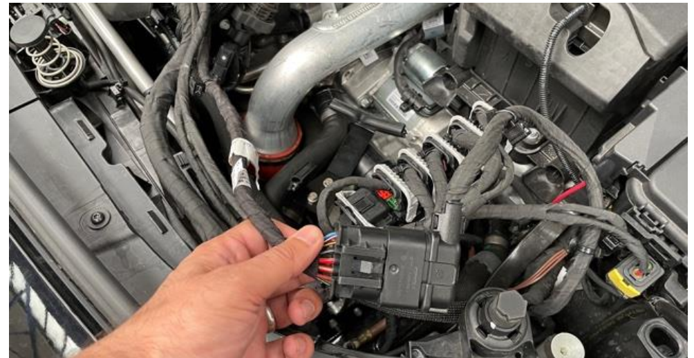
16. Reroute the terminal which was unplugged in step 7. Place the ECU as shown with the plugs facing upwards. See next step for the reroute position.
