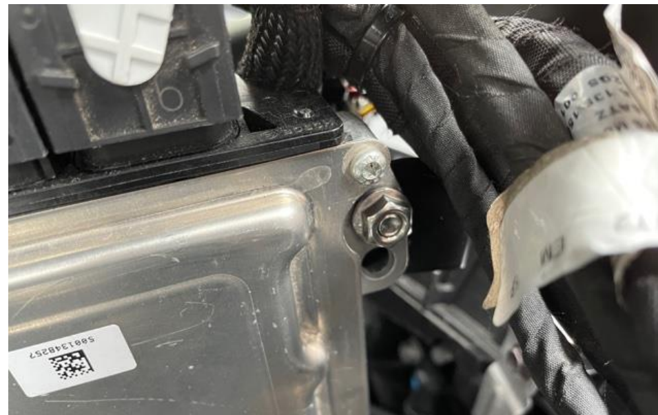
20. Secure this side with an M6 nut and M6 Bolt as shown. Use the upper hole on the ECU tab.
