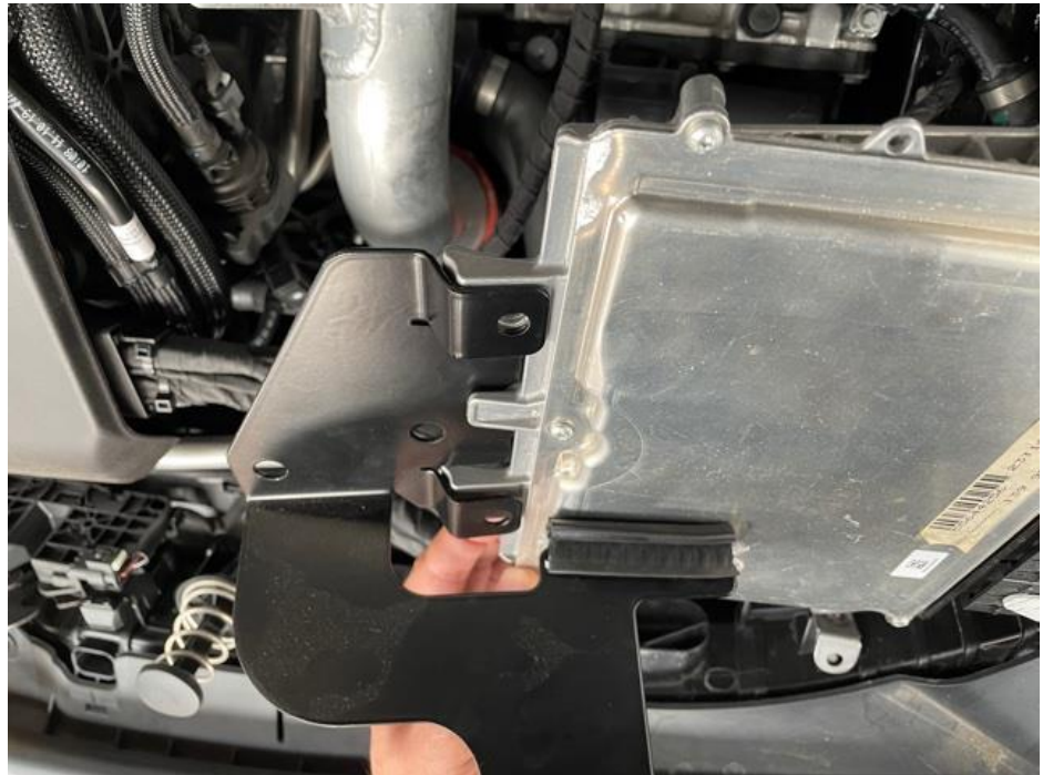
13. Slot the ECU into the bracket as shown. The 2 tabs on the ECU should line up with the holes in the bracket. See next photo for another angle. The circled holes are where this bracket will mount to the chassis in the same position as the stock bracket removed in step 9.
