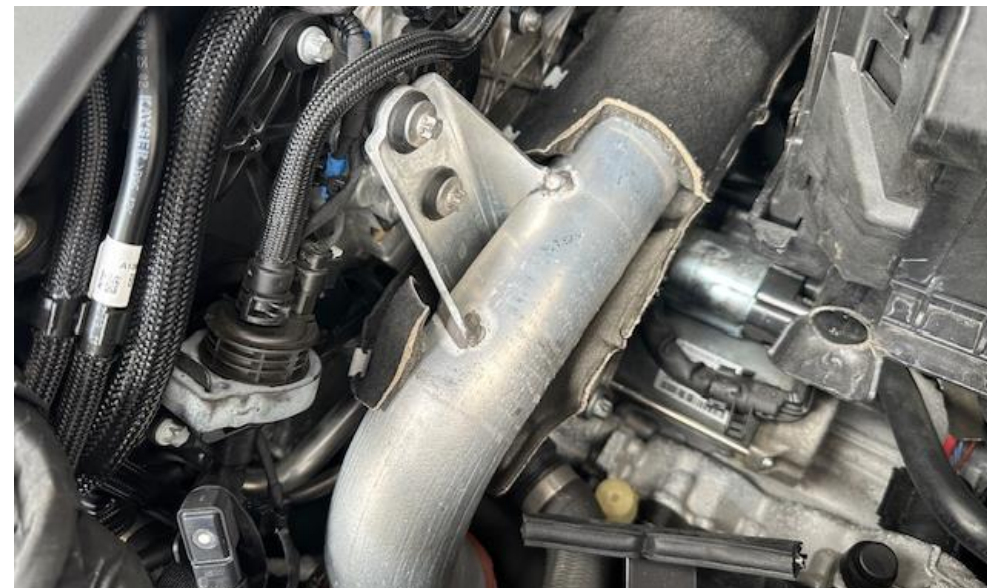
8.5. Remove that piece of insulation as shown. This allows the correct clearance for the new filter housing.
