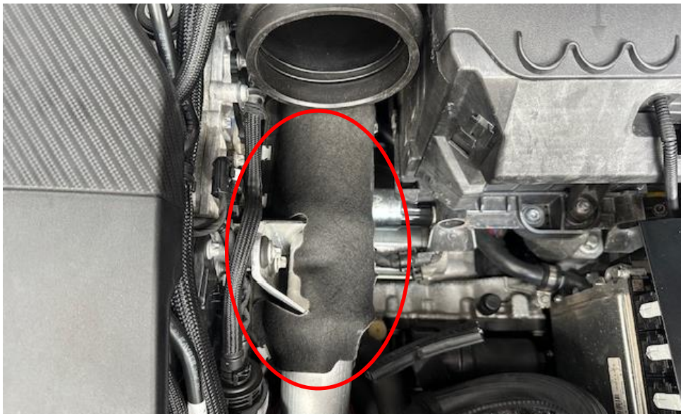
8.2. If the chargepipe under the airbox has an insulating cover as shown – you will need to cut a section out.
