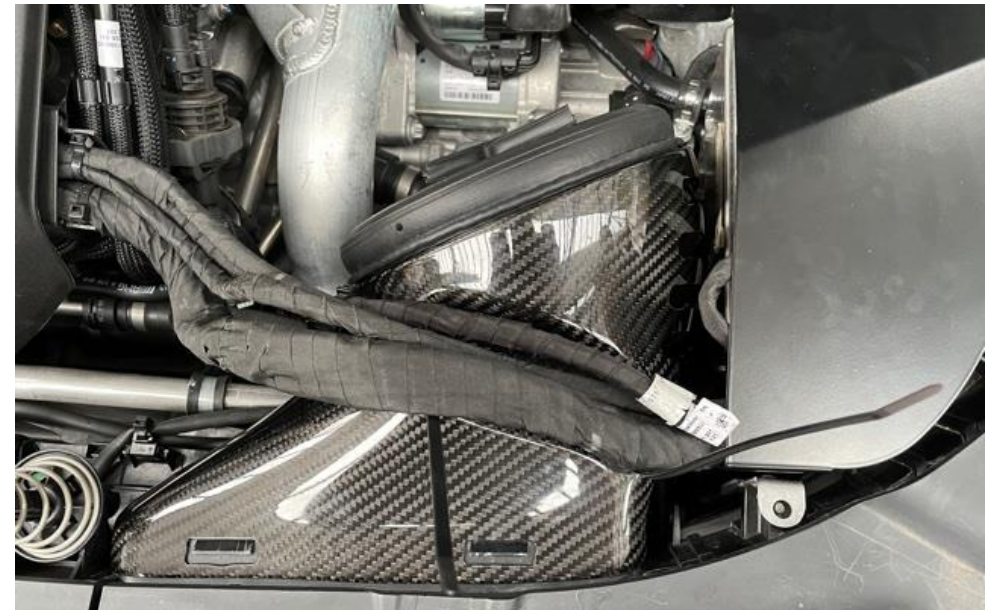
26. Push the carbon duct into place.
