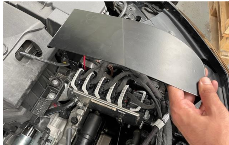
18. Take the cover panel and place it on top of the ECU. See next steps for positioning.
