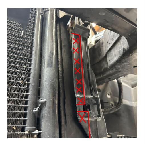
**Modification #4:** Trim the lower right corner of the radiator shroud as marked in the photo.
