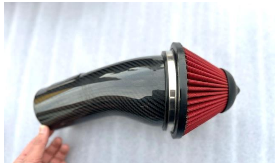
20. Install the filter onto the MAF tube and secure the clamp. Do not over tighten as the carbon can be damaged.
