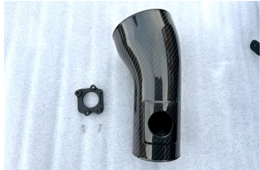
18. Take the Carbon MAF tube, MAF Boss and 2 wide pitch cutting screws as shown in the next step.
