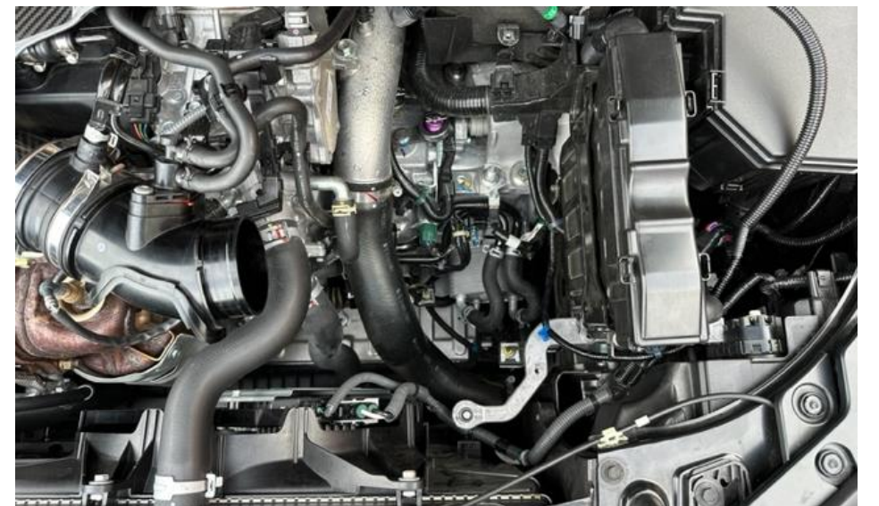
8. Airbox can now be lifted out – there will be a rubber grommet holding it down at the front. It just needs to be carefully pulled out.
