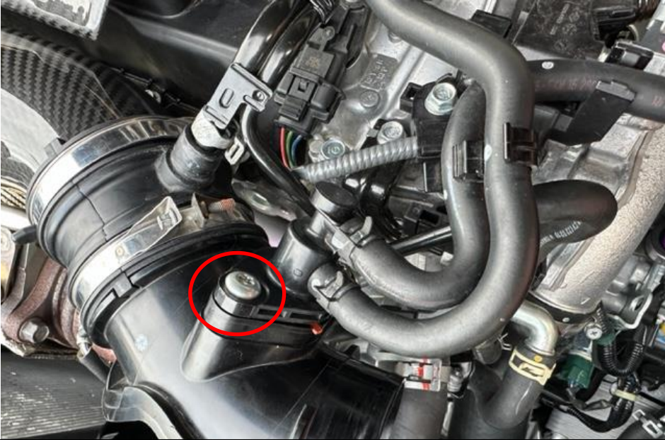
9. Remove the 2 T30 Torx Screws holding the breather module onto the intake tube. These screws will be used again.
