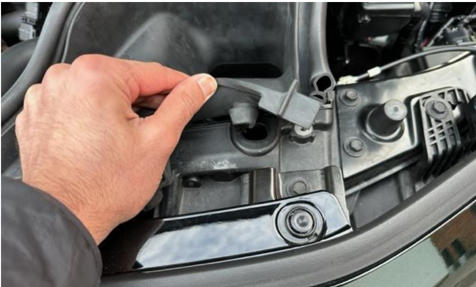
7. Lift the front rubber section of the airbox and carefully pull the moulding out of the slam panel.
