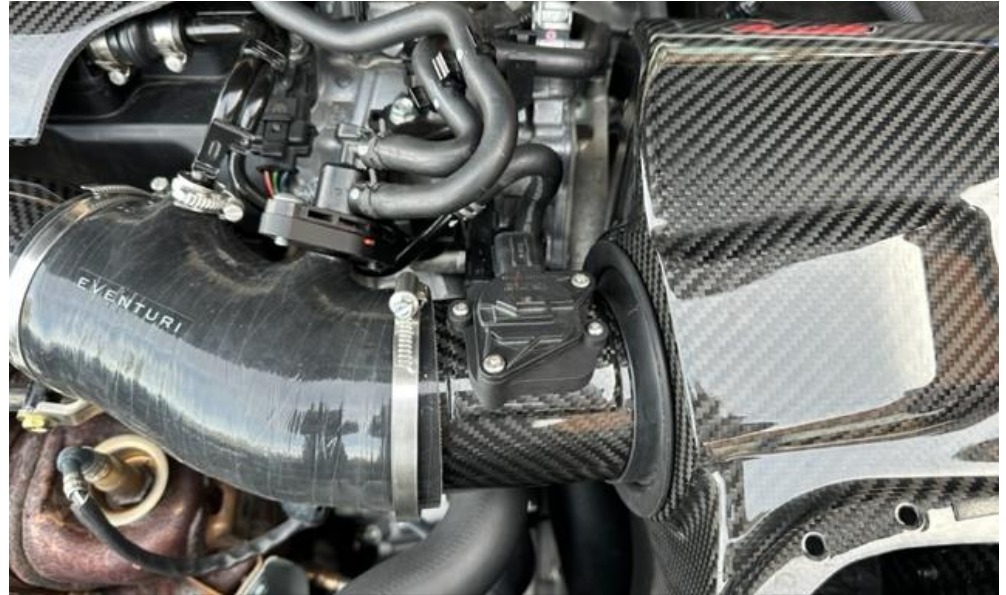
34. Push the MAF tube into the silicon hose. Rotate so that the MAF sensor plug points downwards slightly.
