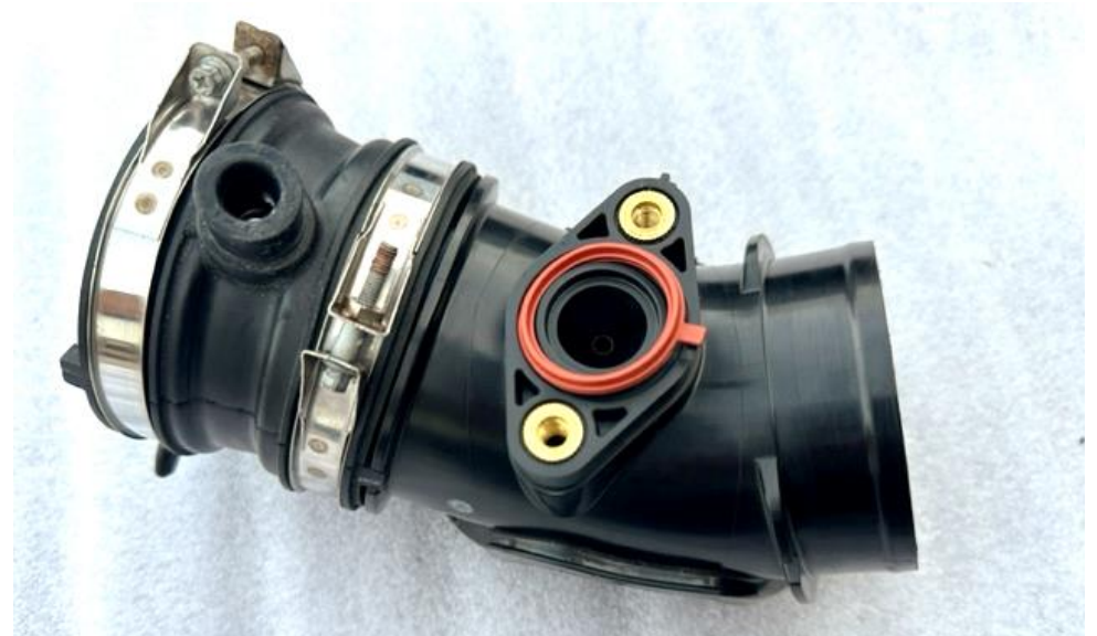
26. Remove the orange rubber seal from the OEM inlet tube.
