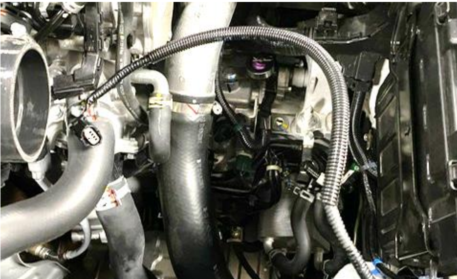
C. Take the supplied cable conduit and cover the exposed MAF wiring with it.
