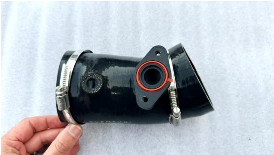
27. Install the orange seal into the new machined mount which is part of the new silicon hose.
