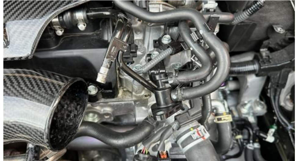
12. Loosen the clamp around the Turbo Inlet tube and remove the OEM intake tubes.
