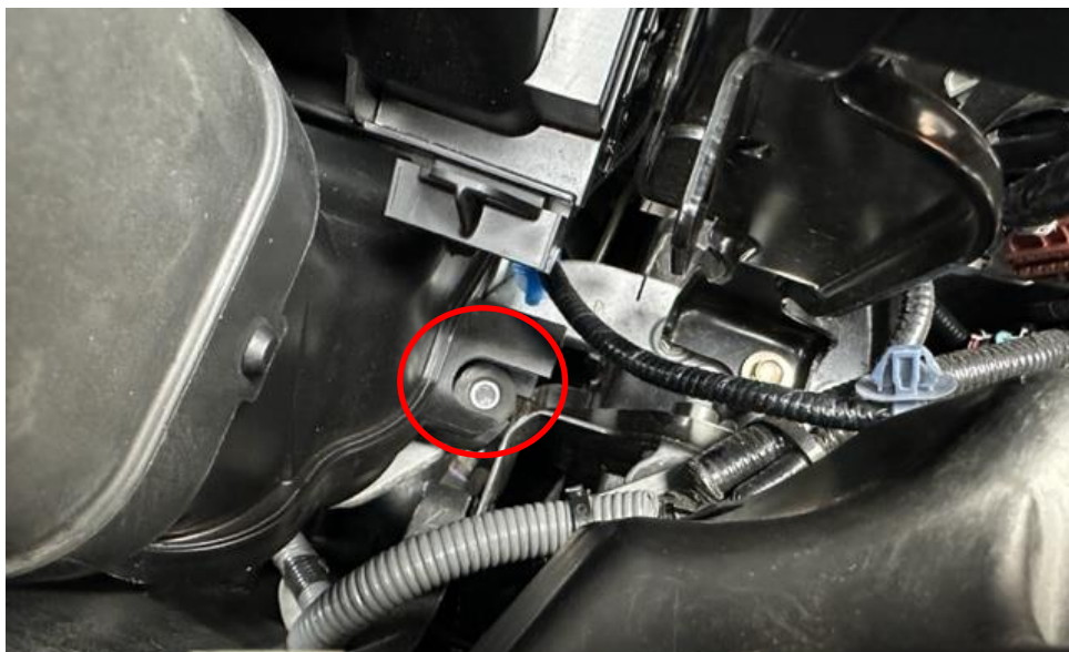
3. Remove the bolt at the front right side of the base of the airbox.
