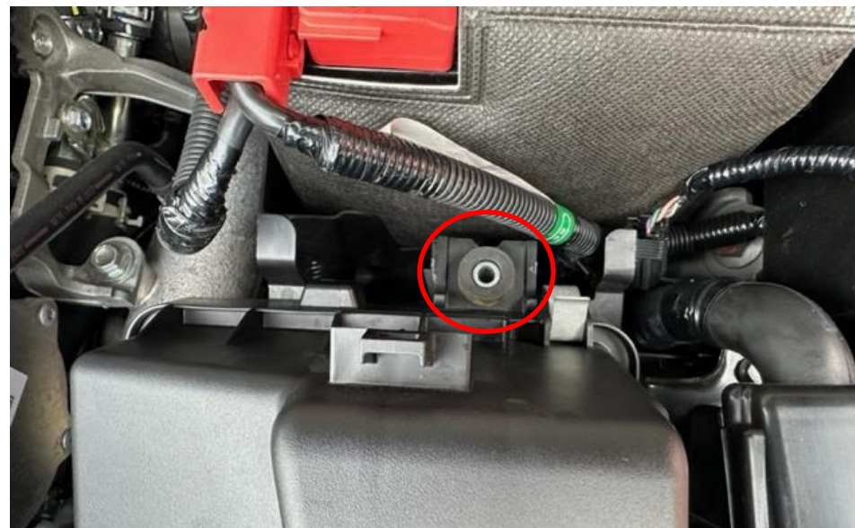
4. Remove the bolt at the rear of the airbox.
