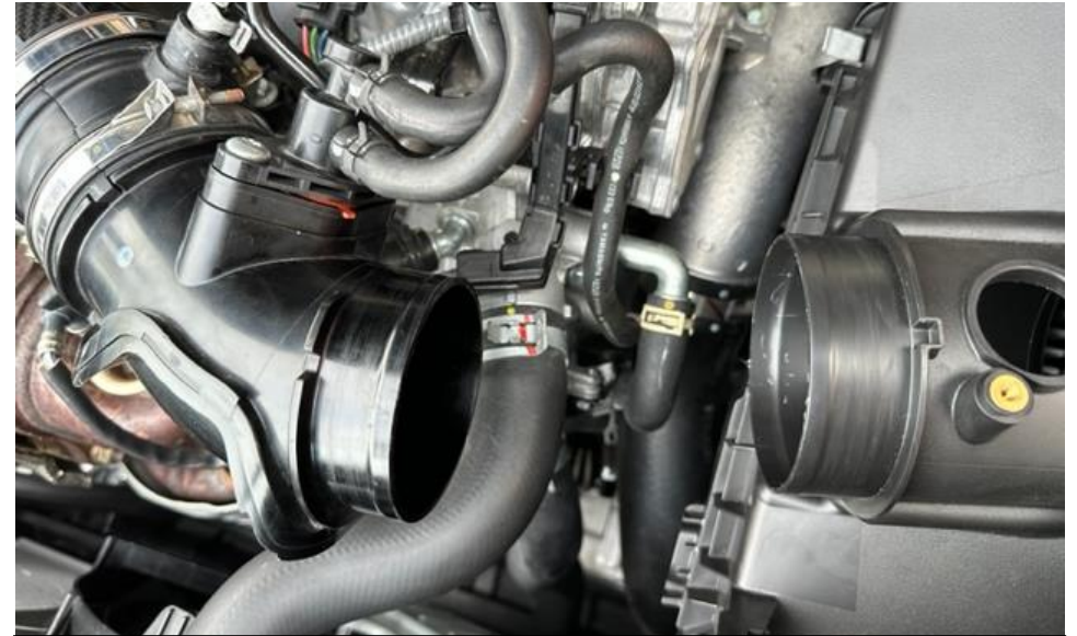
6. Loosen the clamps around the flexible hose and remove it completely.
