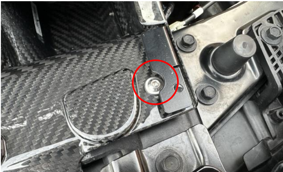
39. Secure the front of the airbox with the supplied 4mm Hex screw as shown.
