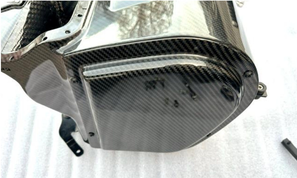
25. Secure the carbon lid to the airbox with the M5 Screws. Do not overtighten.
