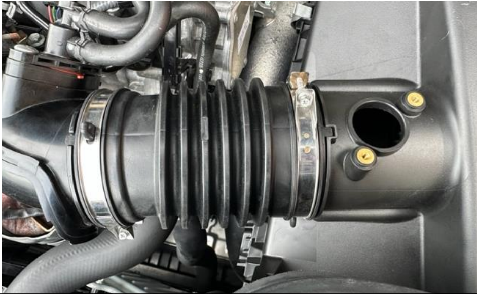
5. Unscrew the 2 screws and remove the MAF Sensor from the airbox.
