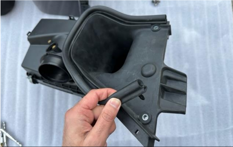
17. Carefully remove the rubber seal from the top of the OEM airbox. It has plastic clips which need to be pulled away from the airbox top.
