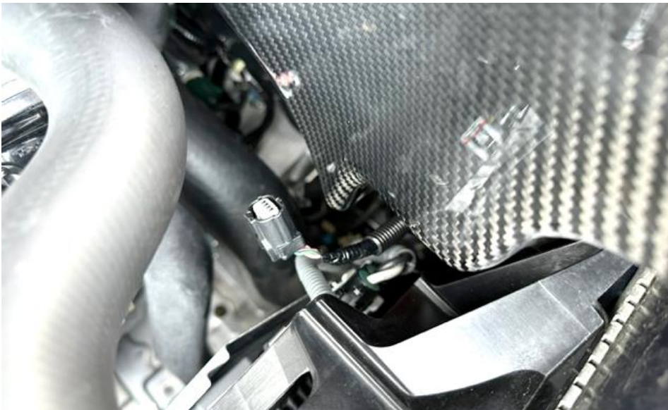
35. Feed the MAF wire and plug under the front of the airbox.
