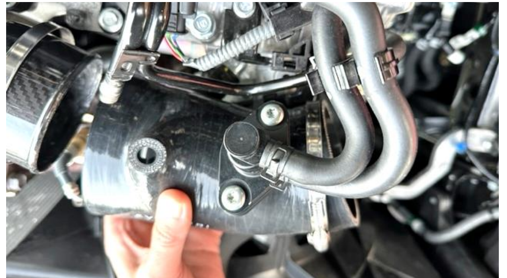
28. Secure the breather module onto the new mount using the T30 OEM screws previously removed.
