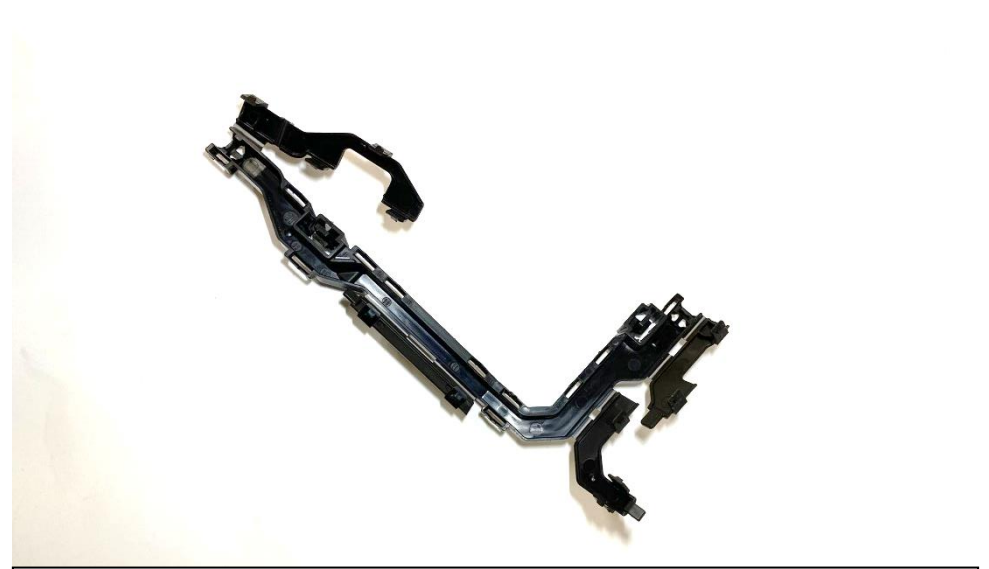
B. Using a small flat head screwdriver, carefully prise open the plastic shroud around the MAF Sensor wire. Here is the shroud once opened and removed.
