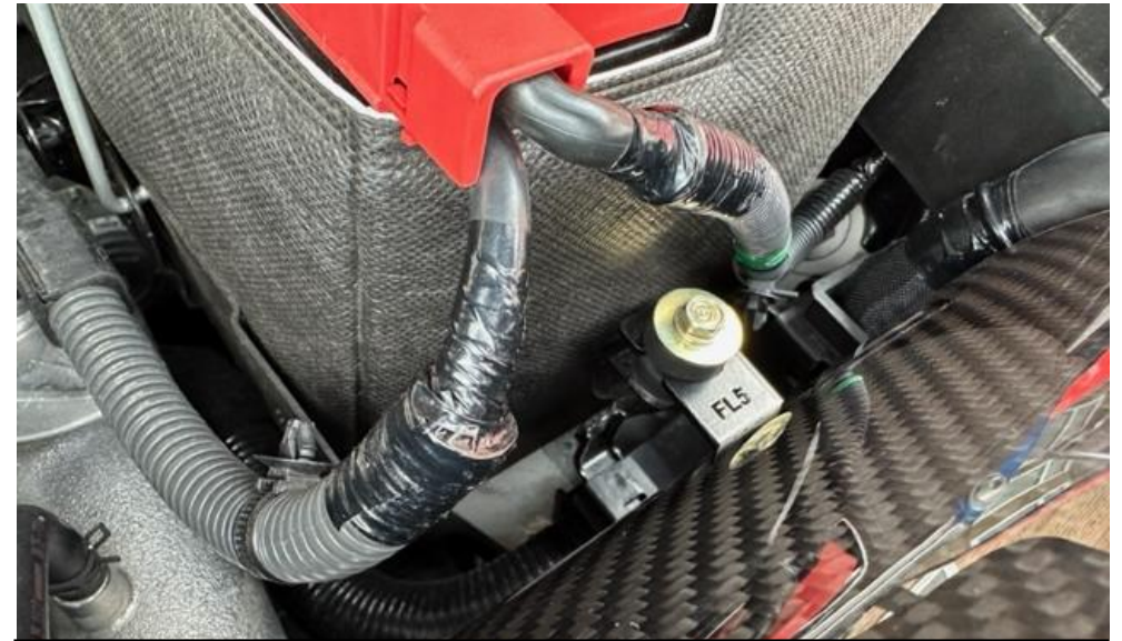
40. Use the OEM screw removed previously to secure the rear bracket of the airbox.
