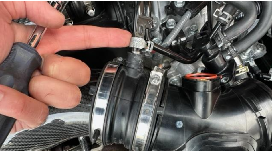
11. Using pliers or a spring clamp tool, lift the small clamp around the metal breather tube away from the rubber hose.
