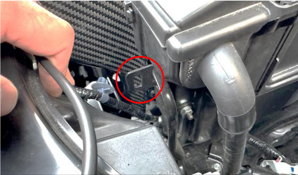
37. Secure the MAF wire by pushing the plastic clip around the wire into this location where the ECU housing is located. (Right side of the airbox)
