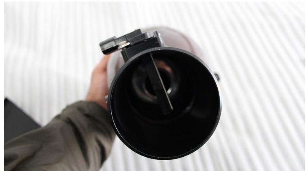
23. Orientation of the MAF sensor with the metal badge on the housing facing upwards.
