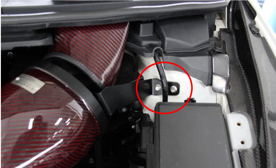
24. Position the bracket which is attached to the housing over the 2 threaded holes on the arch DO NOT secure with the supplied bolts yet.
