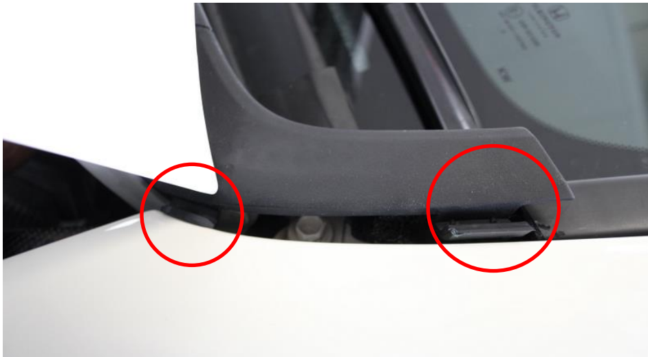
14. Now take the supplied plastic panel which has been pre-cut and install by firstly clicking the side tabs into place.
