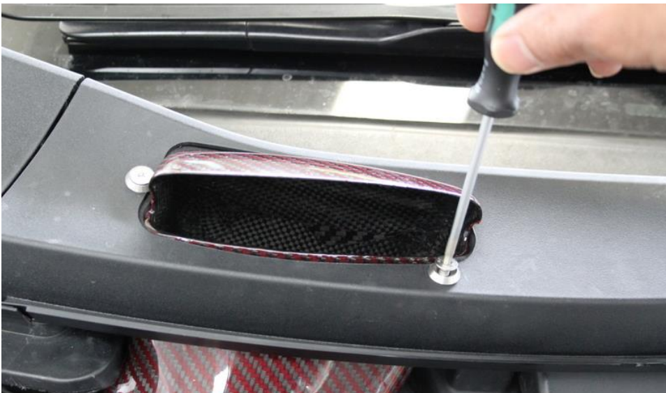
18. Position the duct to line up the threaded inserts with the holes on the panel and secure with the supplied screws. Do not over tighten them.
