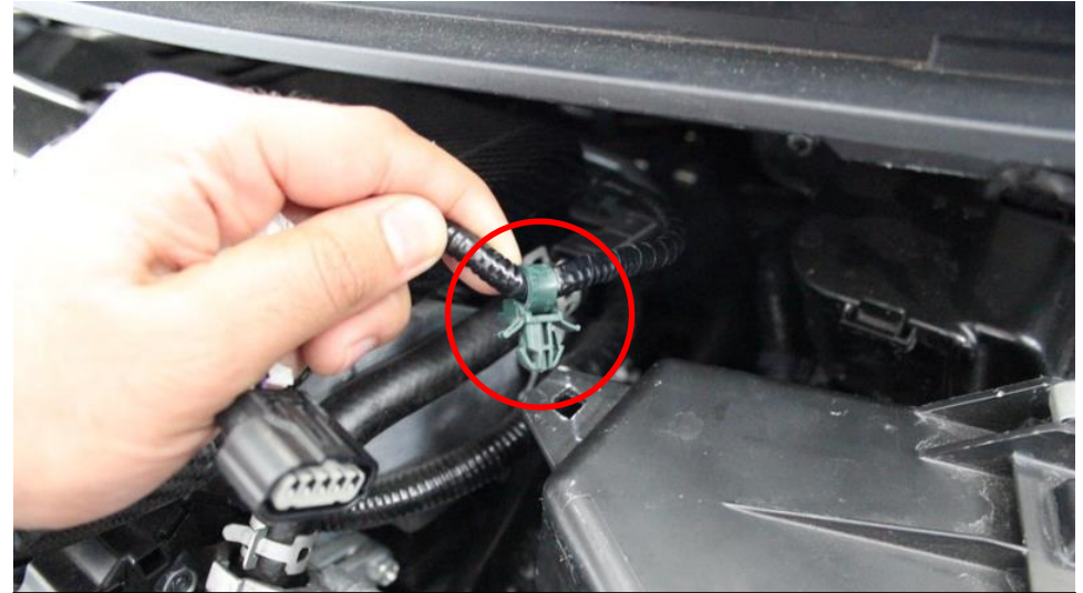
2. Remove the sensor wiring harness from the airbox – push the green tabs inwards to allow you to pull the clip out.
