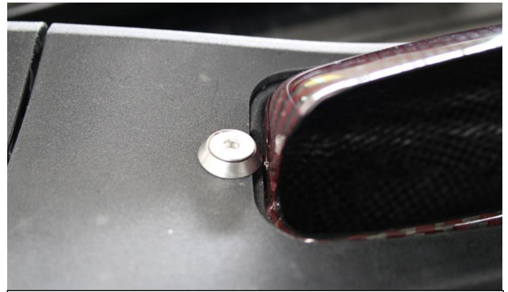
19. Be careful with the left side screw, push the washer away from the duct as you tighten to avoid scratching the carbon.
