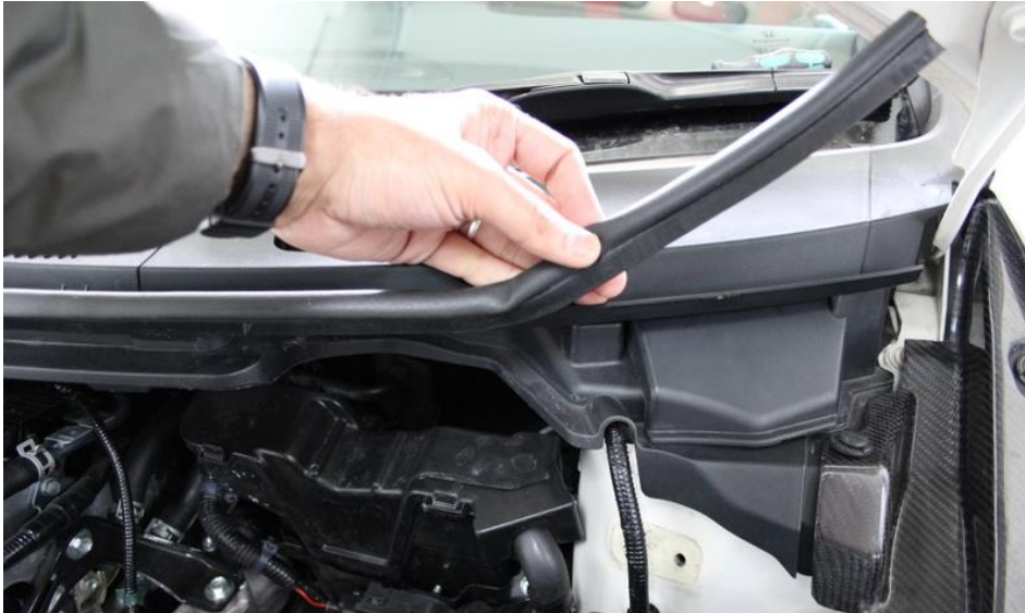
8. Pull rubber trim off the left side plastic panels in front of the windscreen. The left one as you look at the engine.
