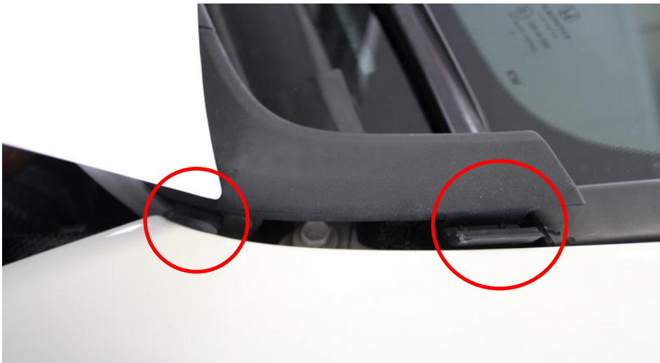
10. Unclip the 2 tabs holding the panel into the wing. Push the panel down to unclip them.
