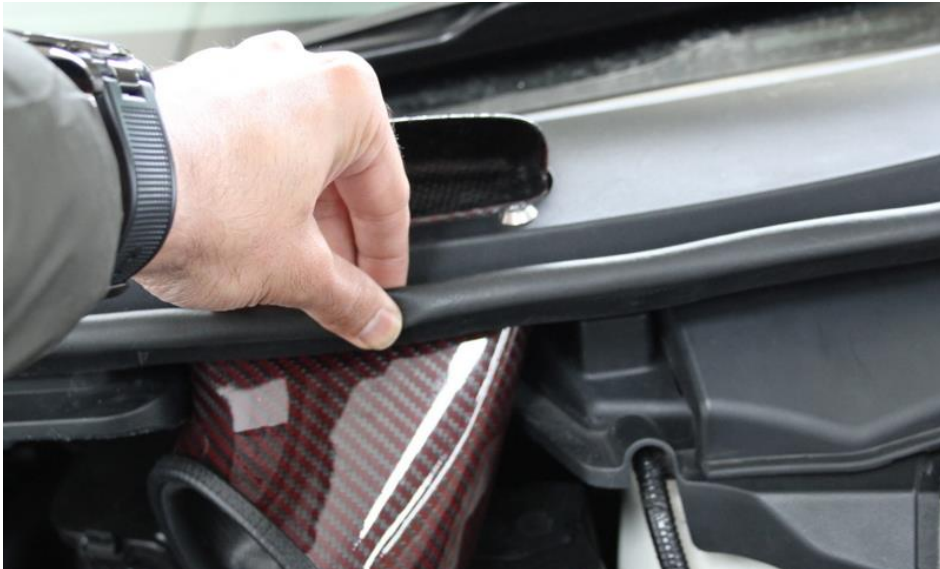
20. Push the rubber trim back into place.
