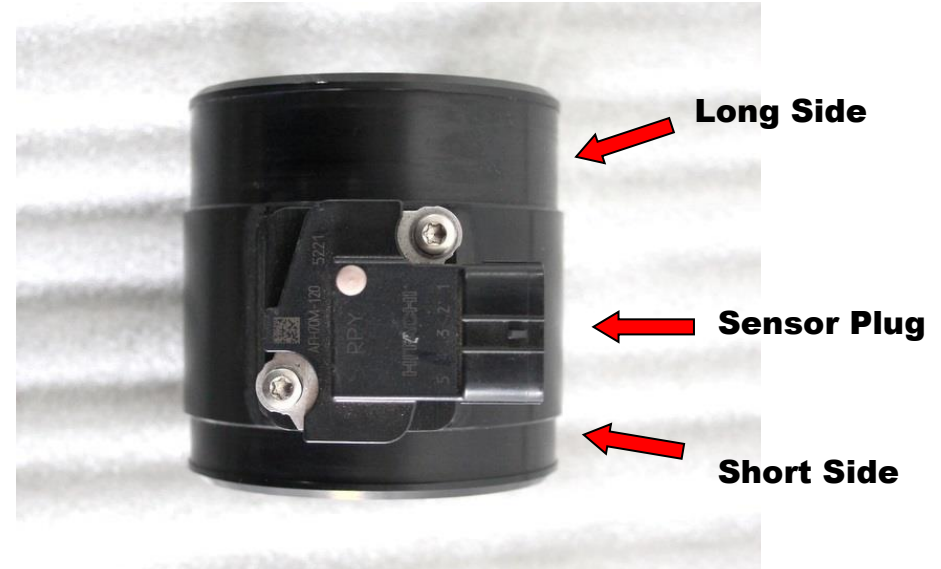
21. Install the MAF sensor onto the supplied sensor tube as shown with correct orientation. Secure with the two supplied M4 screws.
