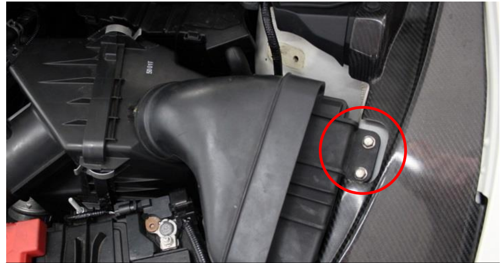
4. Remove the 2 10mm bolts from the intake duct.
