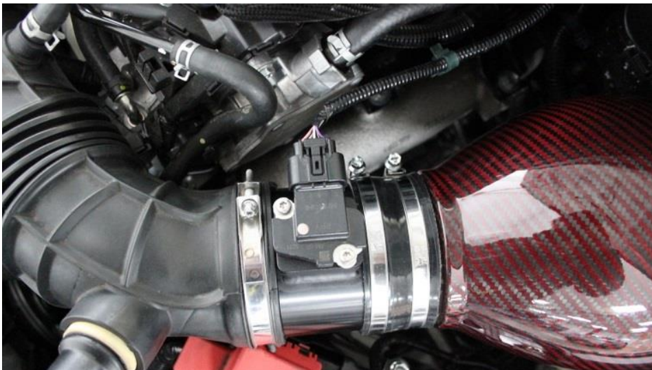
26. Tighten the hose clamp around the rubber tube. Click the MAF sensor plug into place. If the MAF sensor wire is tight, loosen the hose clamps around the silicon coupler and rotate the MAF tube further to give the wire slack.
