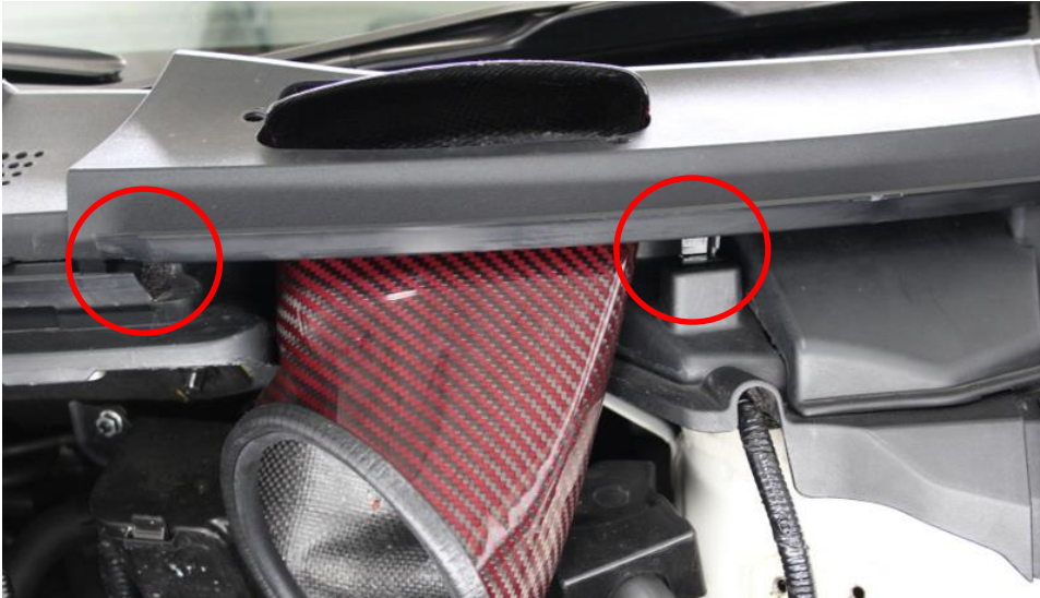
16. Now click all the tabs into place – make sure they go into the correct positions. There are tabs at the back too. Push the panel down all around to click into place.
