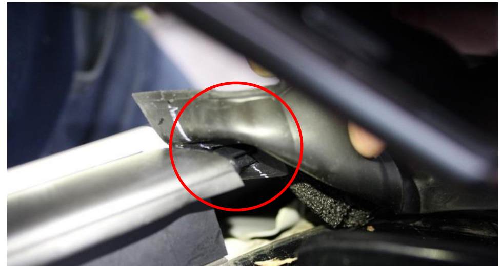
15. Now push the locating tab from the windscreen panel into the hole of this new panel as shown.
