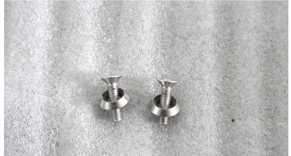
17. We will use the supplied countersunk screws and washers to secure the duct to the plastic panel.
