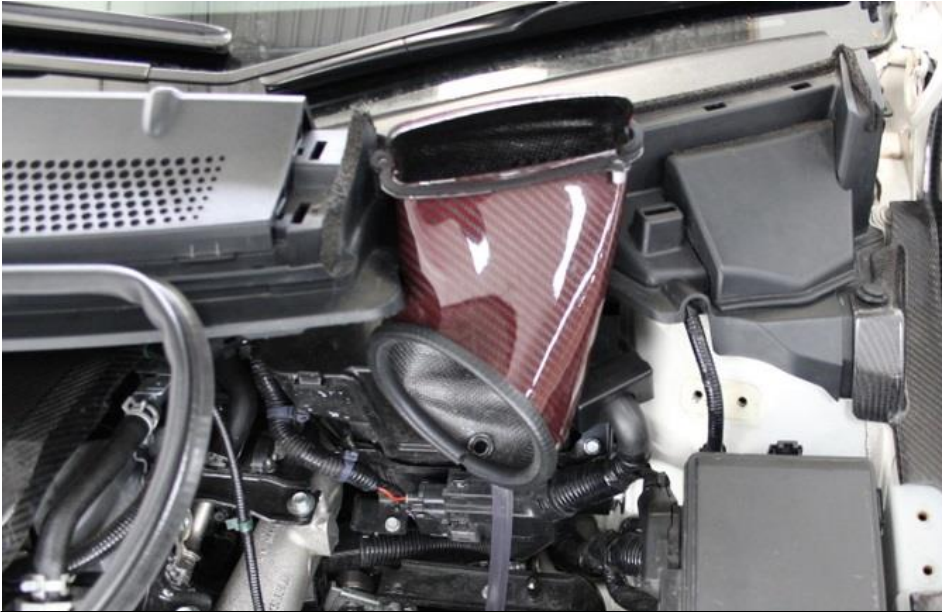
12. Place the carbon duct into the space revealed under the removed plastic cover. This will be secured in the coming steps.
