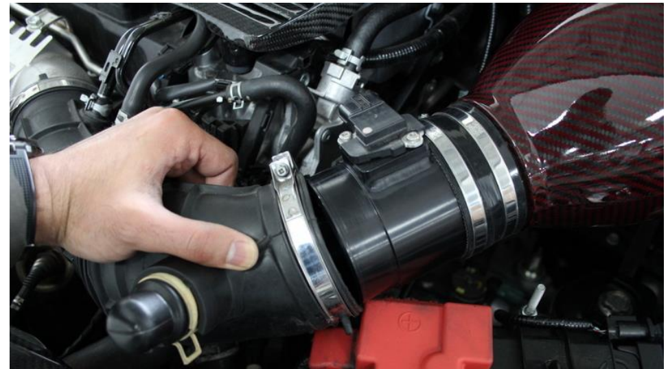
25. Push the stock rubber hose onto the MAF tube – make sure the clamp is loose. Support the housing while pushing the hose on.
