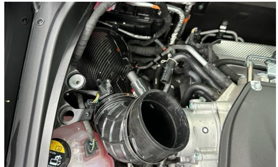
28. Push the flexible side onto the filter housing.
