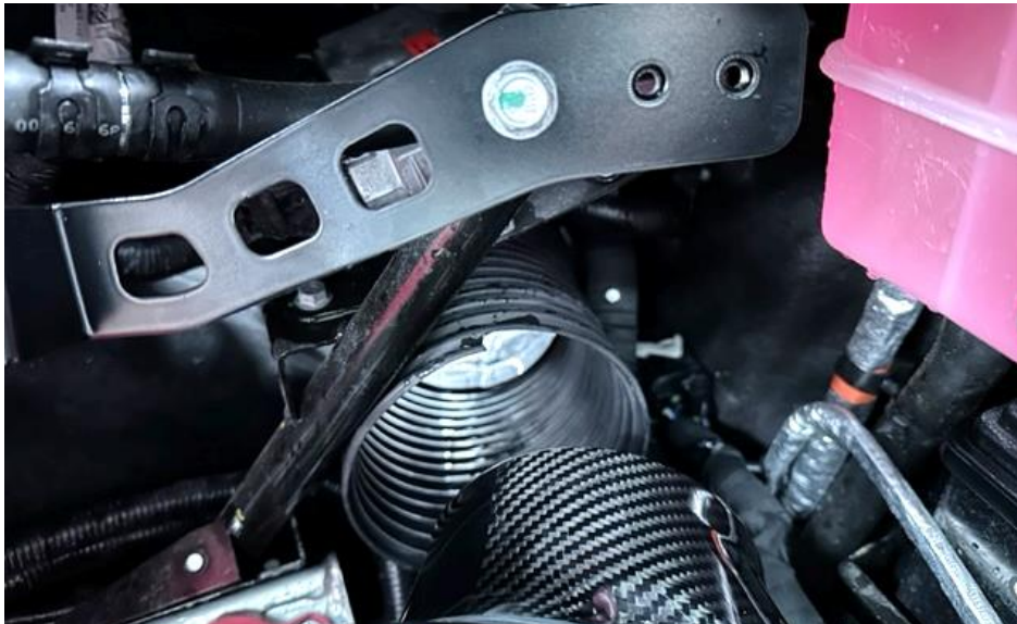
23. The carbon duct needs to be positioned inside the OEM cold air feed.
