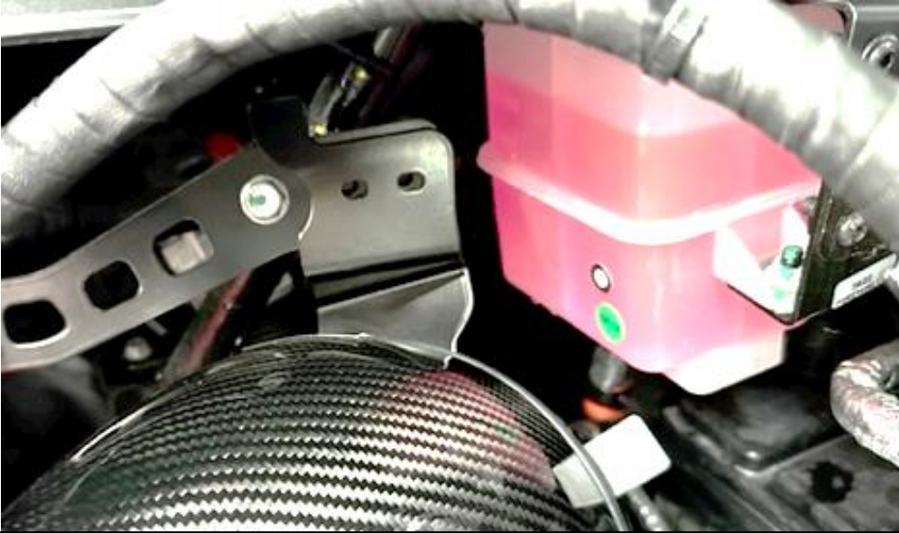
25. Rotate the filter housing to line up the bracket on the housing with the brace previously installed.
