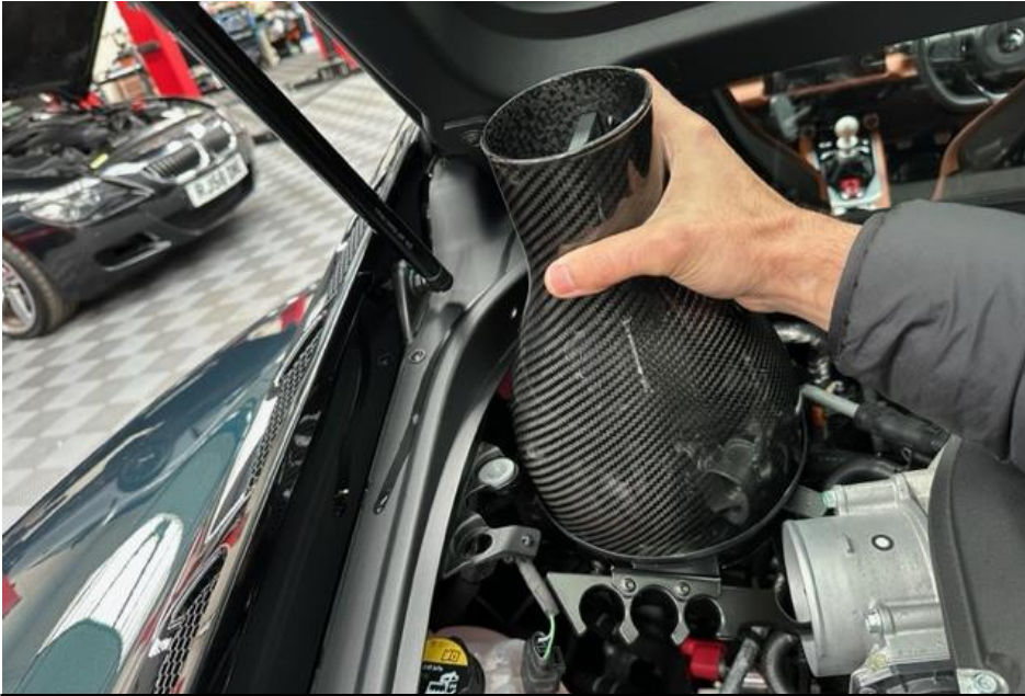
21. Carefully lower the intake into the engine bay.
