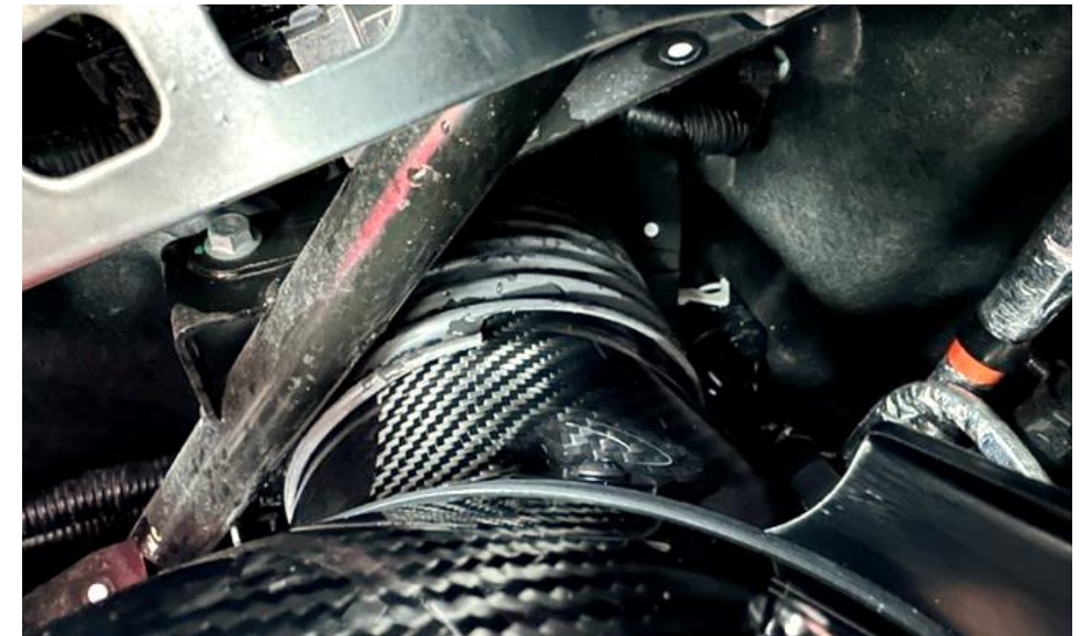
24. Push the carbon duct into the cold air feed.
