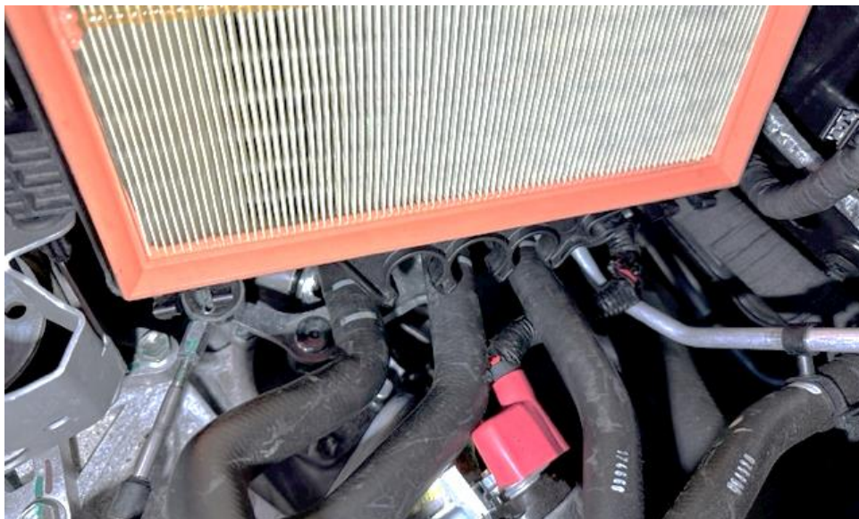
11. Push the coolant hoses off the base of the airbox – pinch them and then push out. Also remove the battery cable from the airbox.
