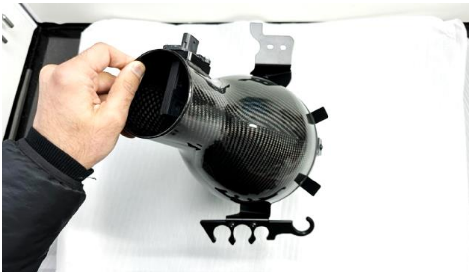
15. Secure the coolant hose holder to the base of the filter housing. See next photo for more details.
