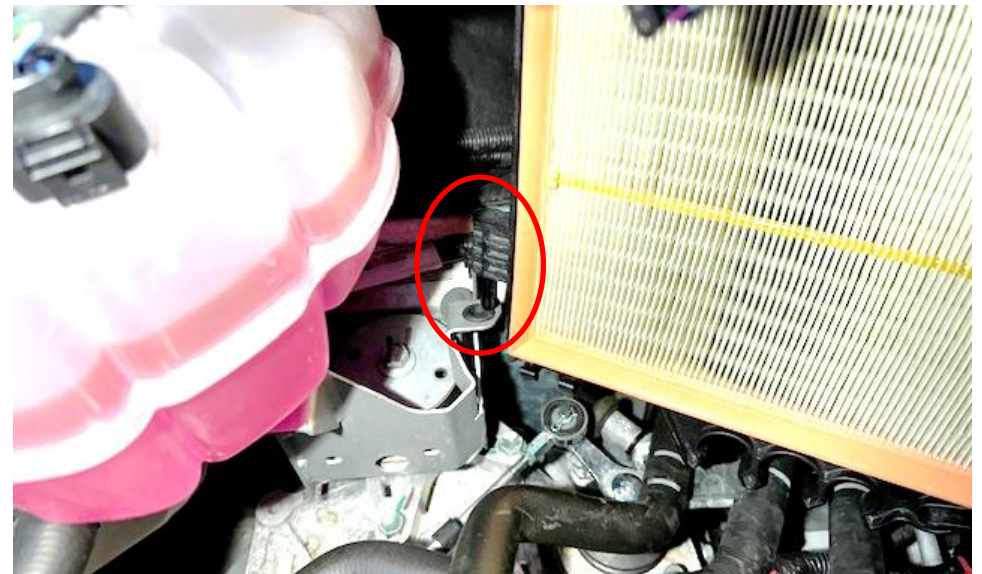
12. The airbox can now be lifted out. It is hooked into place on this side as shown.
