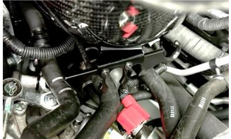
26. Be careful of the coolant hoses at the base – we will push these into the holder after the intake is fully lined up.
