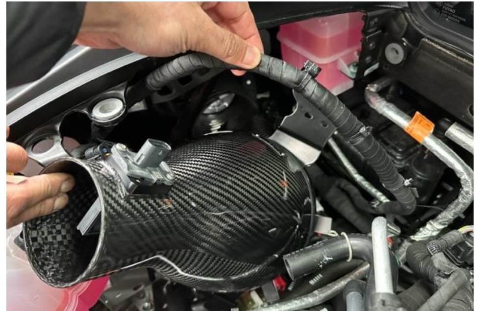
22. Lift the loom over the intake as you lower it into the engine bay.
