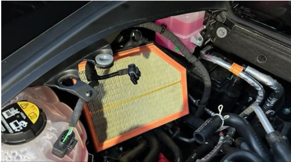
9. Remove the top of the airbox. It will be hooked into 2 points on the base.
