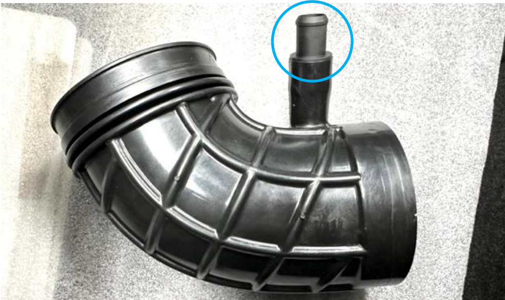
27. Push the breather adapter into the new Flexible Hose. Put the supplied hose clamps on both sides of the hose loosely.
