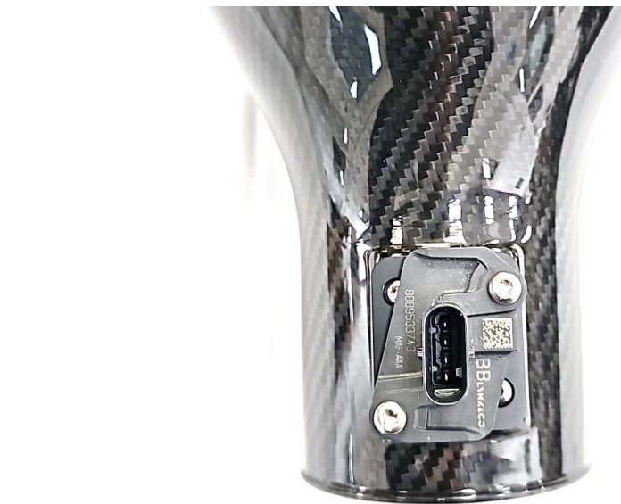
14. Prepare the intake for installation. Install the MAF sensor using the supplied M4 screws onto the carbon filter housing.
