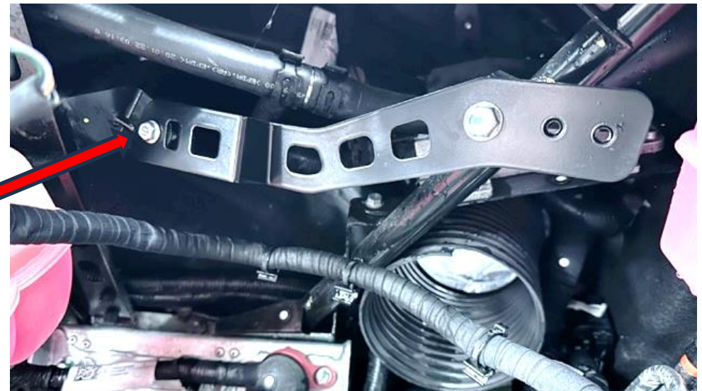
20. Install the brace as shown. M6 Nut and bolt used on the left side as shown. OEM bolt to be used on the right side.
