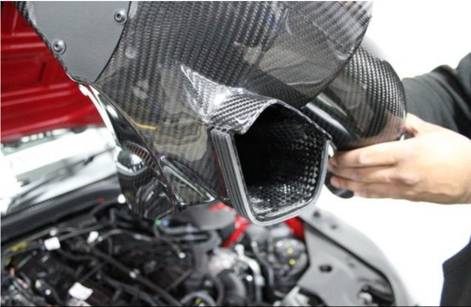
17. The main opening of the airbox should sit inside the stock duct – next photo.
