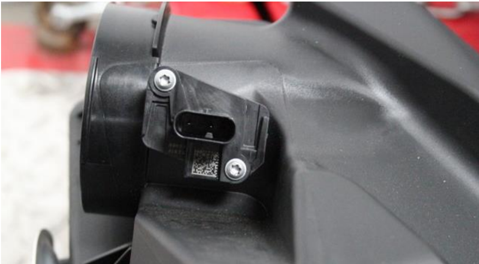
7. Remove the temperature sensor from the airbox.
