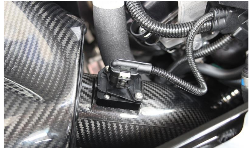
24. Connect the temperature sensor plug.
