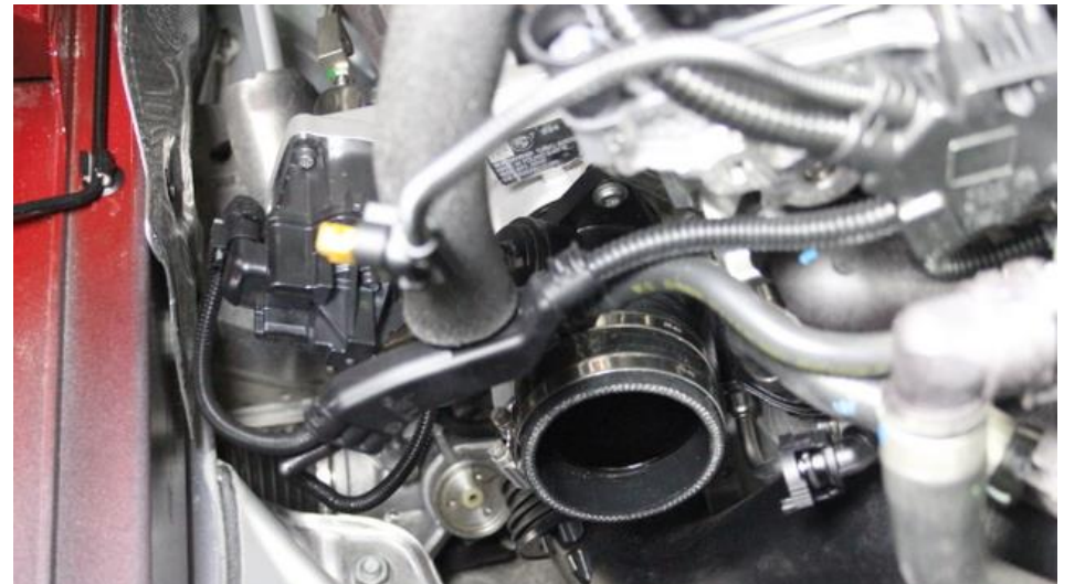
8. install the supplied silicon coupler onto the turbo inlet with the 2 hose clamps. Position the clamp screws so that they are accessible from the side as shown. See next photo for another angle.
