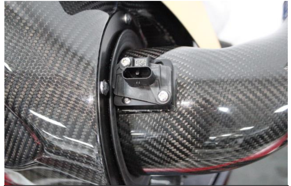
14. Install the temperature sensor onto the tube using the supplied screws. DO NOT use the stock screws.
