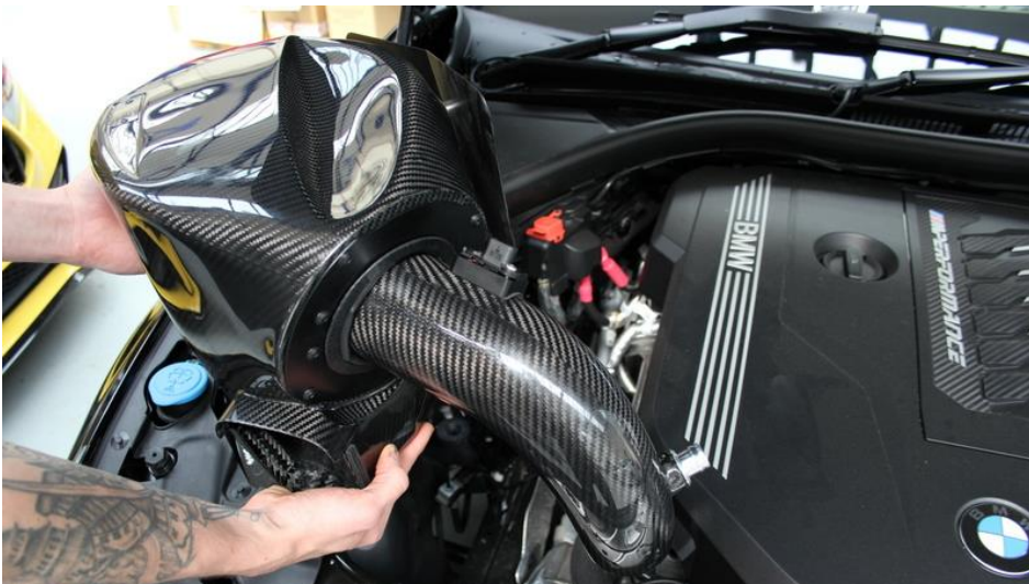
19. Lower the airbox with the tube angled downwards and ensure the mount and secondary scoop go into place as described previously.
