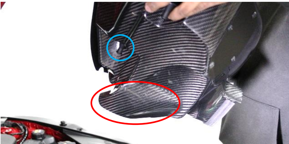
15. Carefully lower the airbox into the engine bay. Note that the secondary scoop circled above goes into the gap shown in the next photo. Also the mount circled blue should sit in the rubber mount shown in next photo.
