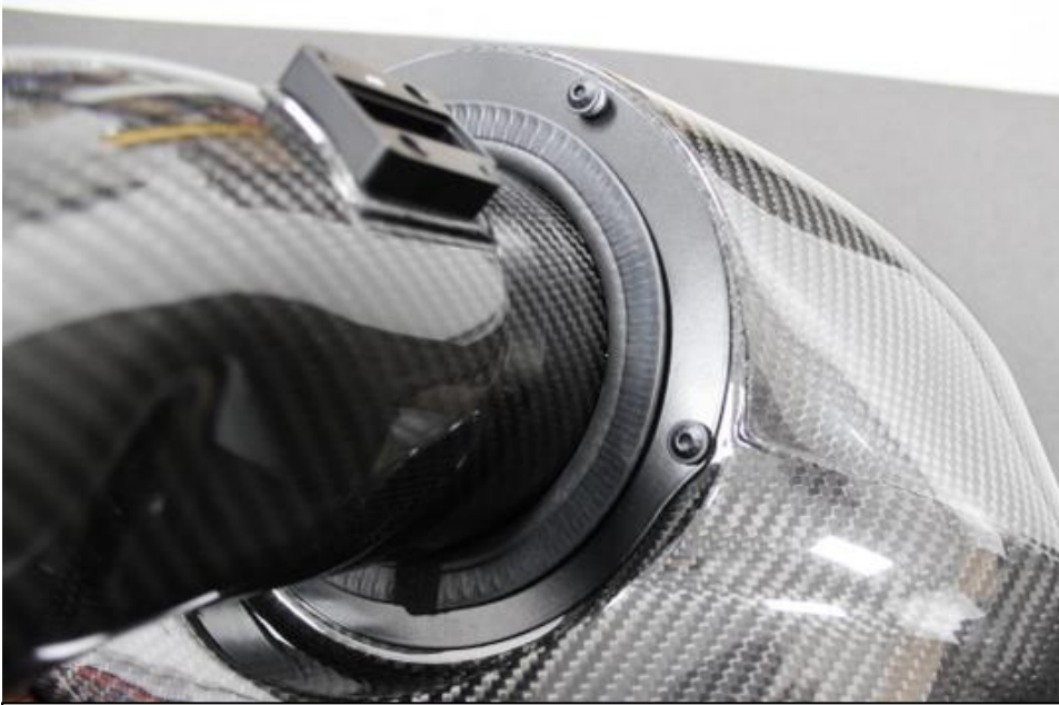
13. Another view of the sealing plate secured to the airbox.
