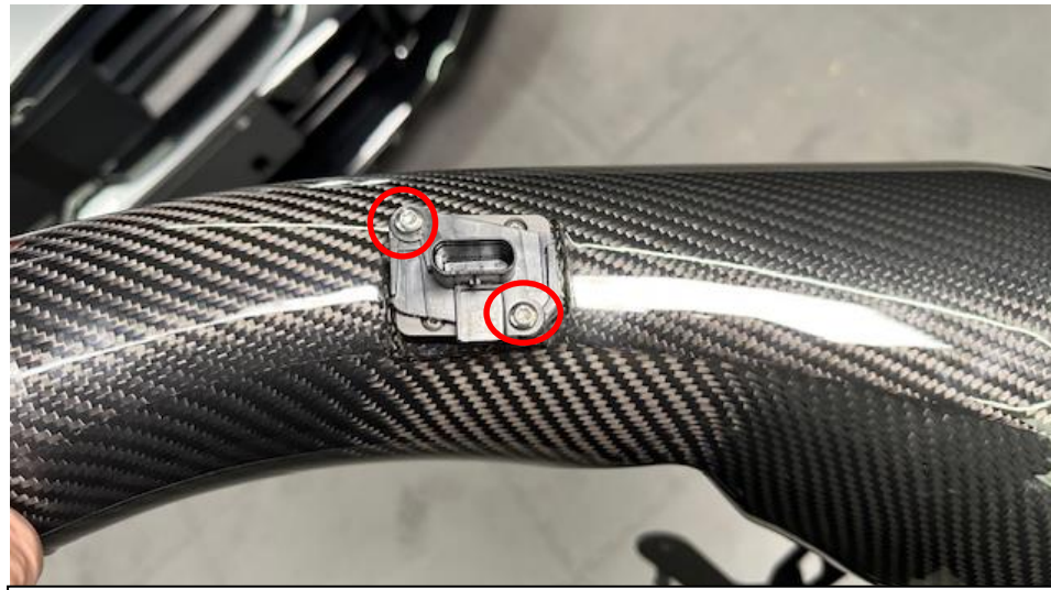
10. Remove the MAF sensor from the stock airbox and install into the Eventuri housing. WARNING – you MUST use the supplied torx M4 screws, not the OEM screws.
