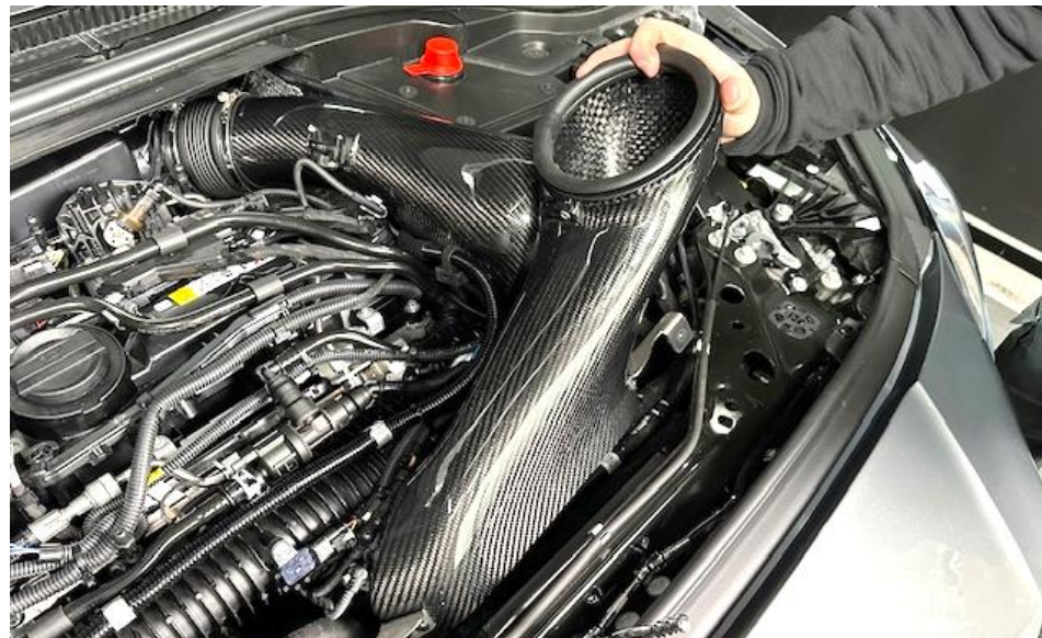
14. Take the duct and start to install the rear of the duct into the OEM air feed at the front of the car. The brackets will go underneath the slam panel. See next step.
