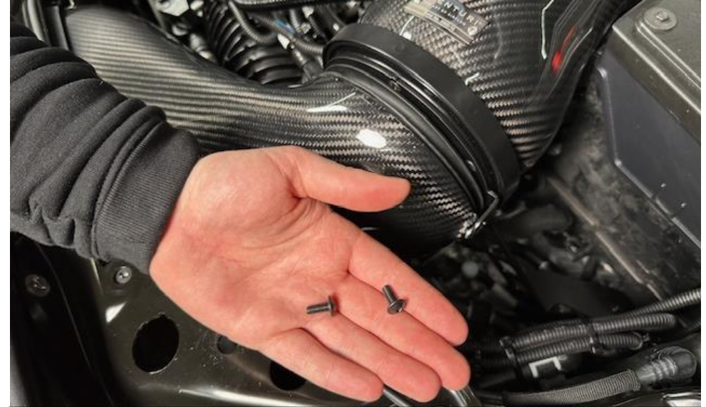
18. Take the 2 supplied flanged hex screws and secure the duct to the housing. See next 2 photos.
