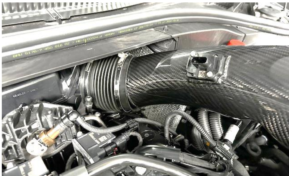
13. Push the Eventuri intake into the flexible hose. Do not fully mount the intake yet. Leave it loose.
