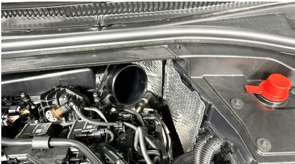
9. Loosen the hose clamp around the back of the flexible hose and remove the hose entirely.
