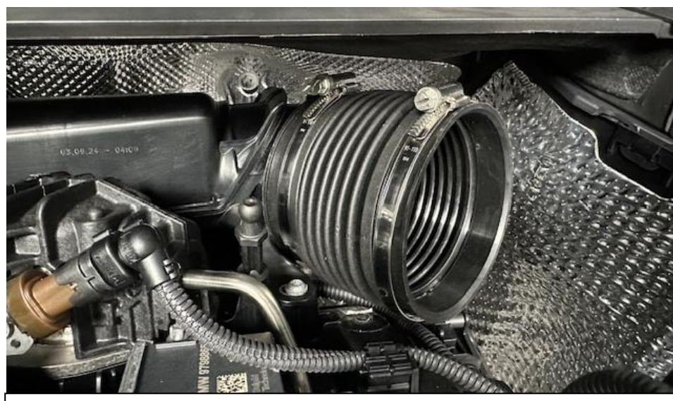
12. Install the hose onto the rear inlet tube using the supplied hose clamps. The F70 TOP side should be facing towards the front of the car. The Eventuri intake will go into that side. Secure the hose clamp on the rear tube.
