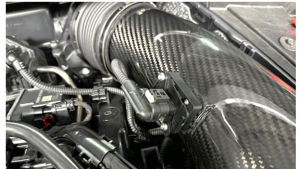
24. Connect the MAF plug into the sensor and lock it with the tab.
