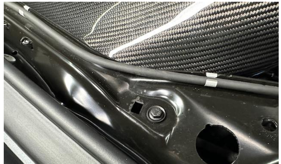
22. Secure the duct using the bolts. The washer will protect the metal. The bolts secure into the duct brackets.
