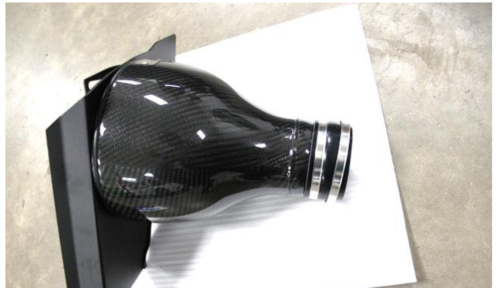
28. Take the LEFT side intake and push a silicon tube onto the outlet as shown. Put 2 hose clamps over the silicon. Clamps should both be 80-100mm size (size is stamped on the clamp). Tighten the clamp around the carbon only.
