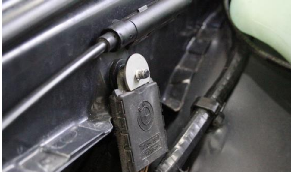
32. Now place the D-Washer over the thread so the flat face is at the bottom as shown.
