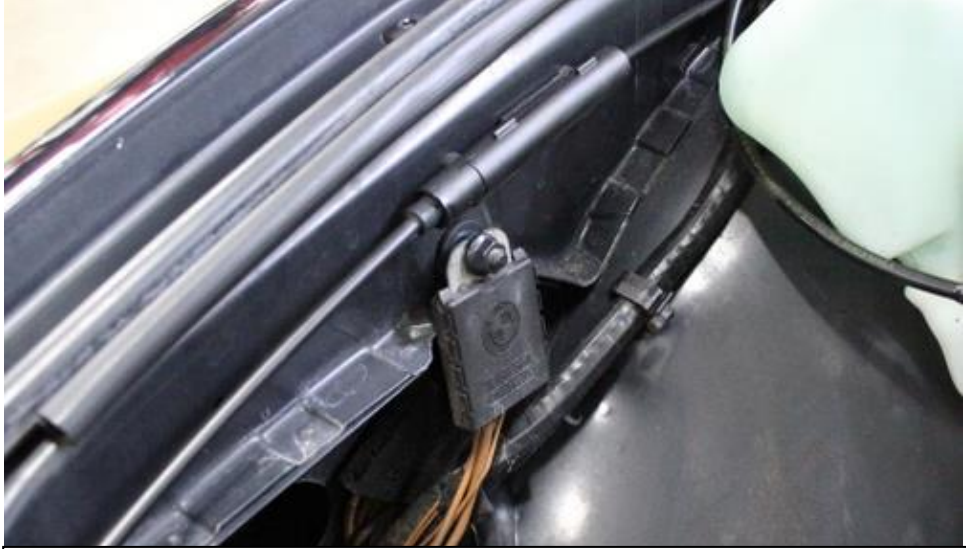
30. Starting with the Left side (LEFT side as you look at the car from the front) Remove the nut holding this sensor in place just above the duct, on the wing.
