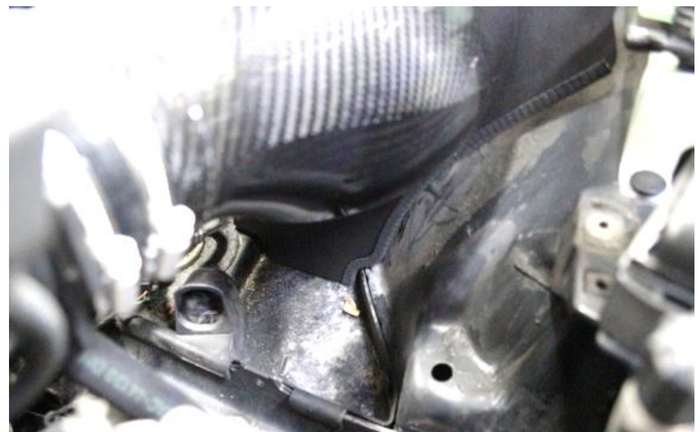
36. The base of the heat shield should slot into place as shown. Photo is showing the rear of the shield.
