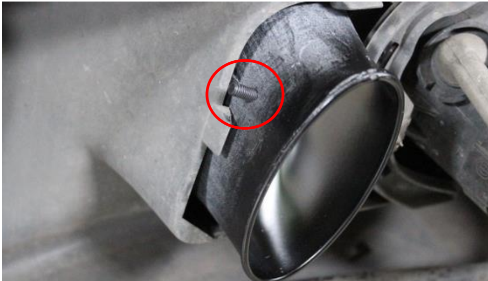
15. Push the M5 screw from the inside of the outlet so that you can see the thread.
