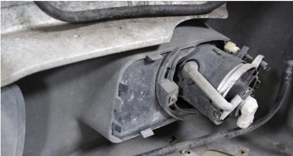
11. We now need to remove the Foglamp surrounds. Start by pushing the clips down from behind the bumper. This should allow you to push the surround out.
