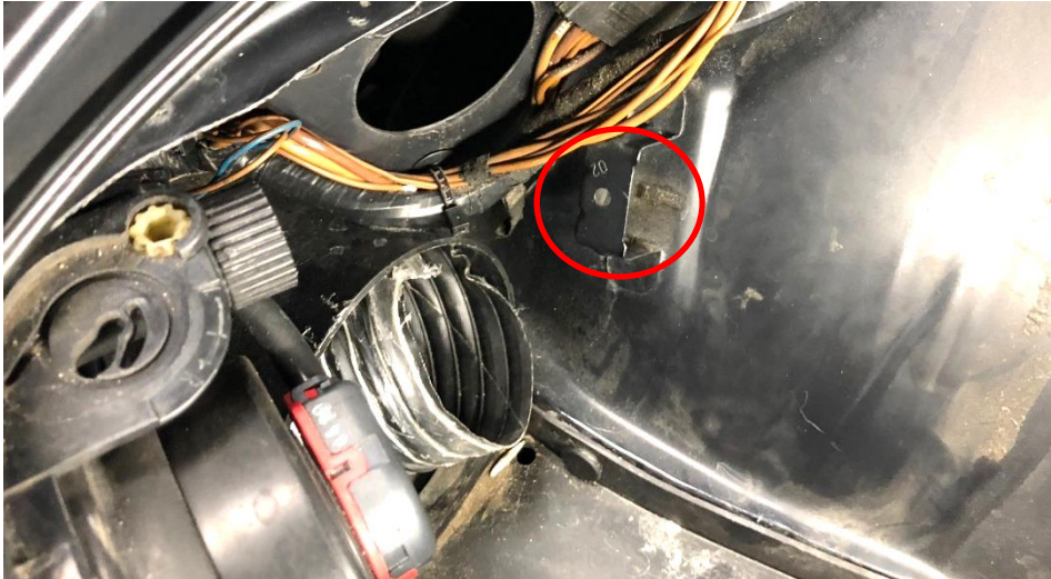
25. Starting with the Left side (as you look at the car from the front) The bracket will secure to the mounting point shown here.
