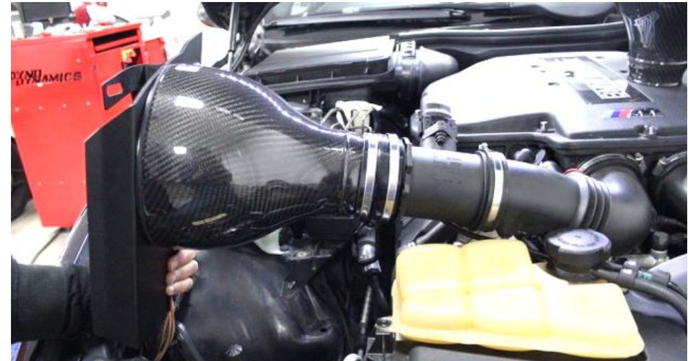
34. Push the LEFT side housing with silicon onto the MAF tube. Do not tighten yet.
