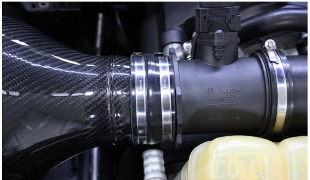
40. Ensure the silicon is sitting squarely on the MAF tube and tighten the hose clamp around the silicon over the MAF tube.
