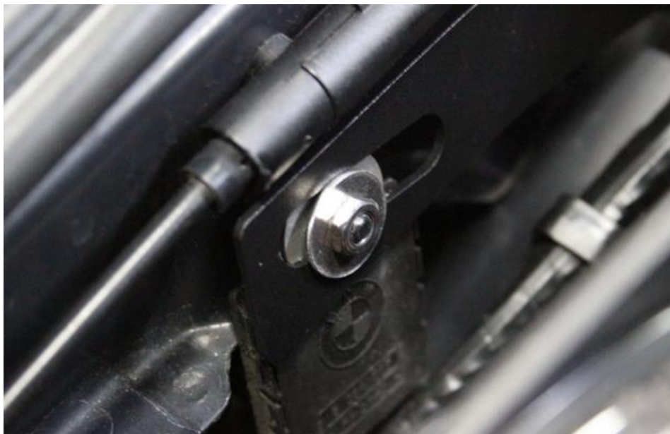
39. Use the remaining Washer and Shallow nut from step 29. Secure the bracket.
