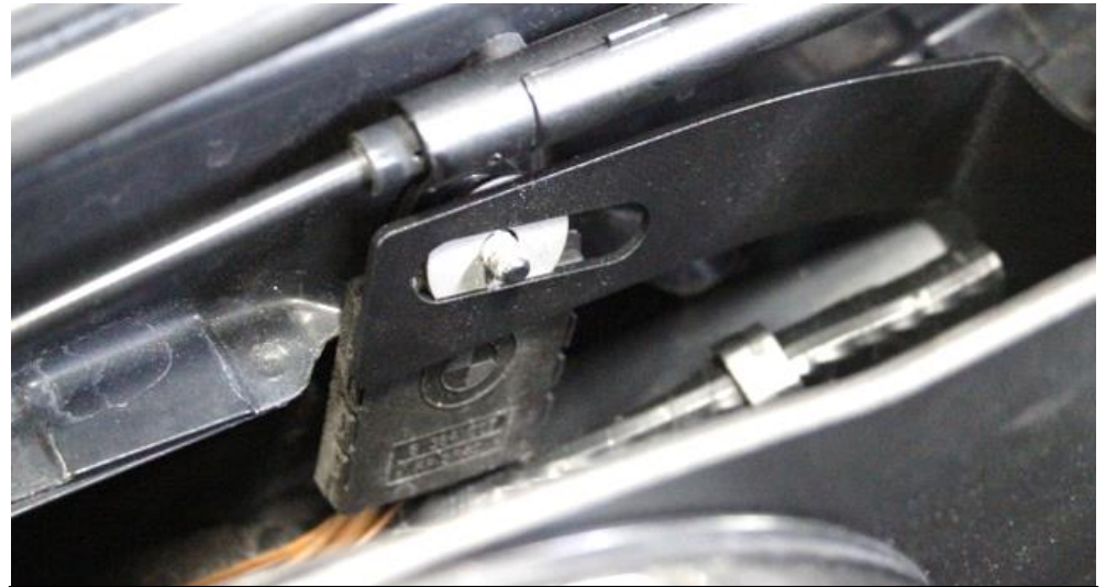
38. Position the bracket so that it sits over the thread securing the sensor. Ensure that the D-Washer over the sensor is still in correct orientation.
