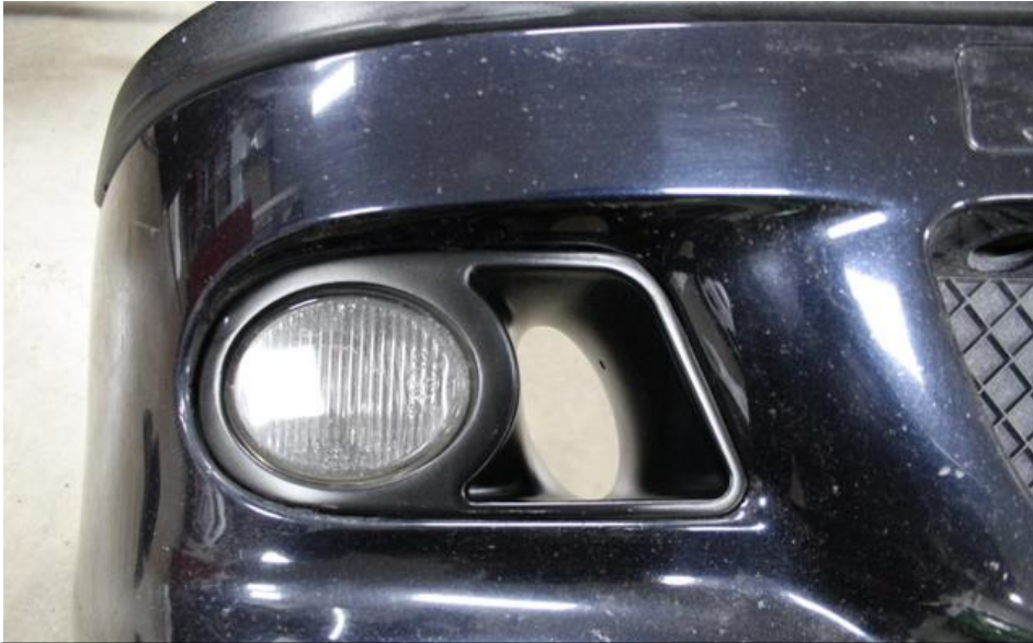
13. Take the new foglamp surround with integrated inlet and push into place.
