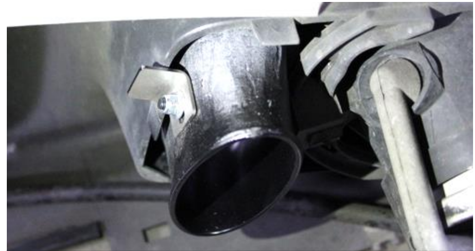
16. Place a bracket over the screw thread as shown with one face towards the bumper edge. Apply the locknut to the screw – use the supplied Allen Key to hold the screw from the inside as you tighten the nut. Do not fully tighten down yet.
