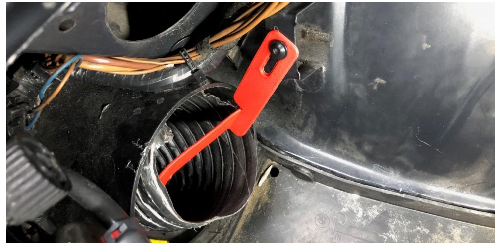
26. Fasten the bracket to the mount as shown using an M6 bolt and nut. The toothed end of the bracket goes into the duct to position it so that it will face the filter. Shown in red for clarity. Do for both sides.
