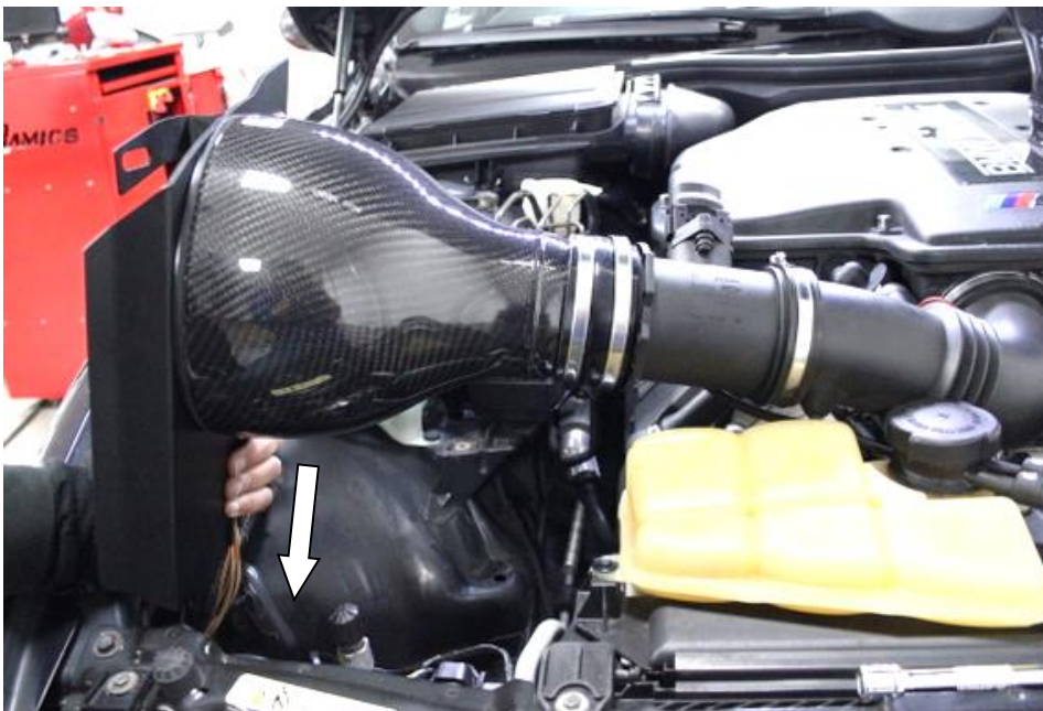
35. Rotate the assembly down while pushing the intake back to get clearance with the wing.
