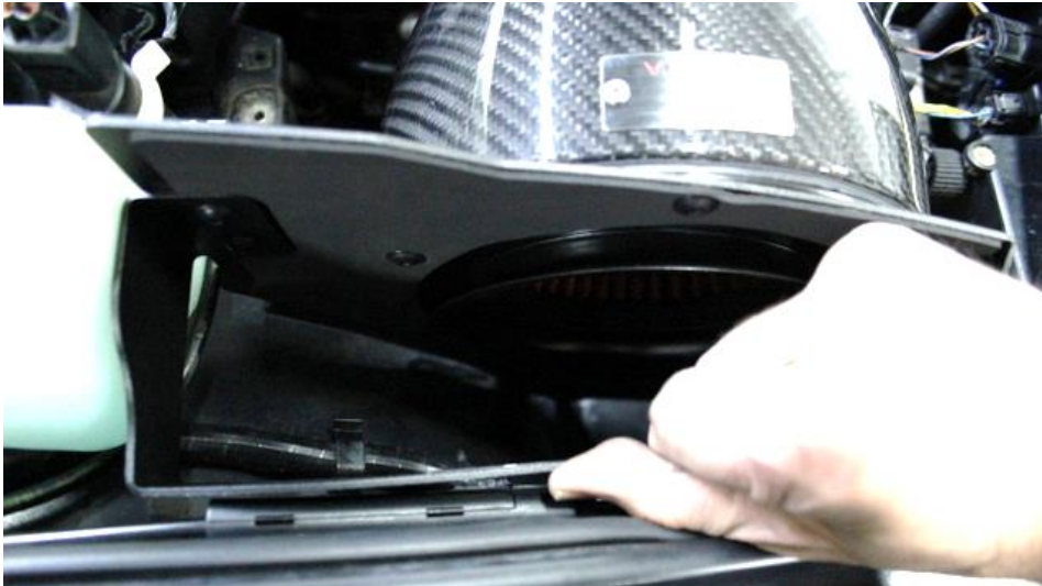
37. As you move the intake down – push back the bracket on the front of the intake to clear the wing. It needs to sit over the sensor – see next step.
