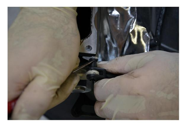
**Step 9** – Remove the two T20 Torx screws securing each of the intake manifold flap sensors to the intake manifold. Remove the sensors to access the intake manifold flap rods. **Do not lose any of them!**
