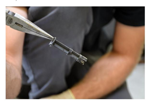
**Step 7** – Locate the factory plastic intake manifold flap linkages. Carefully remove the black plastic pins securing the linkages to the flap actuators.
