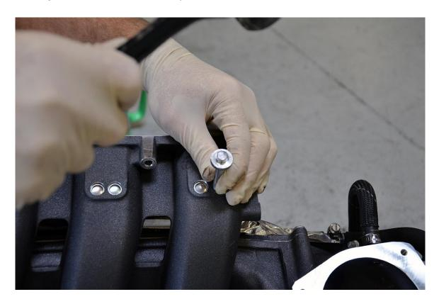
**Step 2** – Continue removing the intake manifold plugs until you've removed all 16 of them. Set the plugs aside for reinstallation later. Pat yourself on the back – you deserve it!
