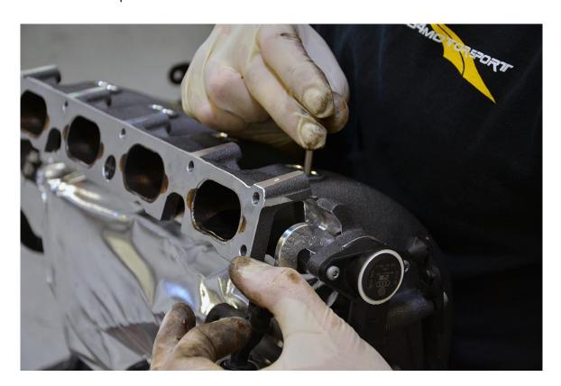
**Step 20** – Apply Loctite to the intake manifold plugs you removed in <u>Step 1</u>, and gently tap them in using the shorter (small) end of the supplied Intake Manifold Plug Installation Tool. **Do not use the longer end for this!** The stop on the short side is designed install at the exact depth necessary for a proper seal. **Pressing the plugs too far in can result in them entering the intake tract!**
