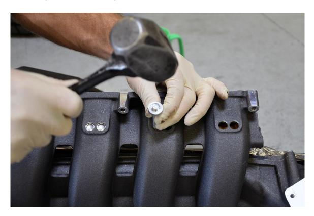
**Step 3** – Locate the T20 Torx screws that are now accessible through each of the holes for the plugs you removed. These secure the intake manifold flaps to the rod, and need to be removed for installation of the billet linkages. Remove them using a T20 Torx driver. There will be 2 for each flap, or 16 in total. **Do not lose any of them!**
