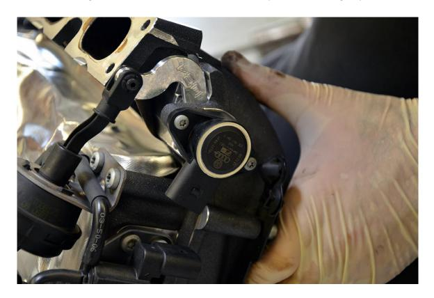
**Step 18** – With the intake manifold on its side, gently place the intake manifold flaps into the ports, aligning the holes on the flaps with the threaded holes in the intake manifold flap rod.
