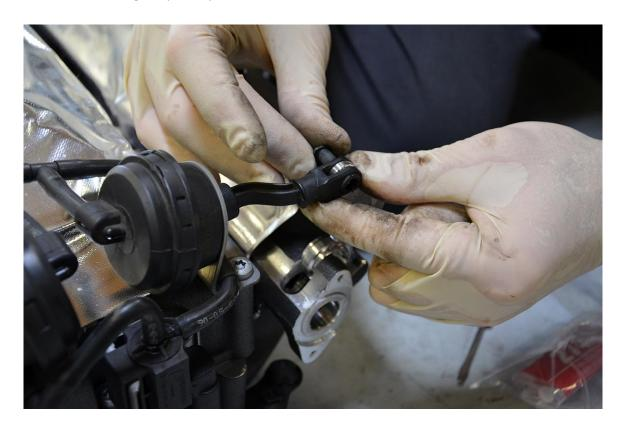
**Step 13** – A set of channel lock pliers may be used to ensure that the plastic pin is fully seated.
