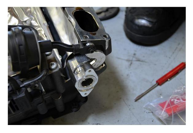
**Step 15** – Once the intake manifold flap rods are installed, check to make sure that they are centered. This is done via the small hole you removed the retaining plug from in <a href="Step 5">Step 5</a>.
