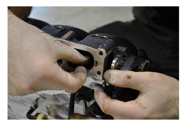
**Step 19** – Apply Loctite to the threads of the T20 Torx screws you removed from the intake manifold flaps/rods in <a href="Step 3">Step 3</a>, and use them to secure the flaps to the rod.
