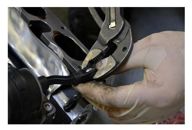
**Step 14** – Align the large end of the intake manifold flap linkages with the slots on the intake manifold, and reinstall the intake manifold flap rods, paying close attention to the orientation of each key to ensure it aligns with the machined keyway on the corresponding linkage.
