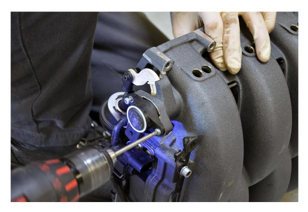
**Step 10** – The intake manifold flap rods can now be **CAREFULLY** pushed/pulled out towards the front of the car, away from the throttle body. You may need to remove the small plugs opposite the flap position sensors for easier removal.
