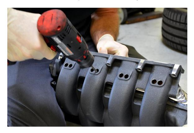
**Step 4** – Remove each of the intake manifold flaps through the intake manifold ports. There are 8 in total. **Do not lose any of them!** You're already keeping track of 40 things you don't want to lose, so give yourself another pat on the back. Excellent work!
