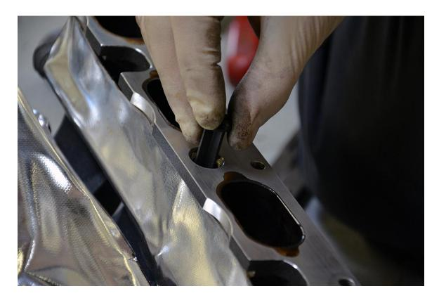
**Step 17** – Reinstall each of the intake manifold flap sensors to the intake manifold, and secure each using two T20 Torx screws. We recommend tilting the manifold on its side to reinstall the flaps in the following step.
