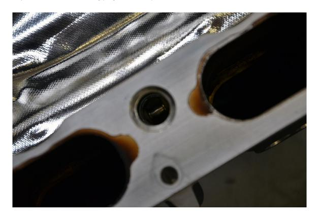
**Step 16** – Verify that the retaining plugs are oriented correctly, and reinstall them into the intake manifold, pressing carefully onto the intake manifold flap rods.
