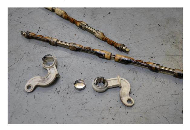
**Step 12** – Begin by installing the corresponding billet aluminum flap linkage to the correct intake manifold flap actuator, as pictured below. Secure using the plastic pin.
