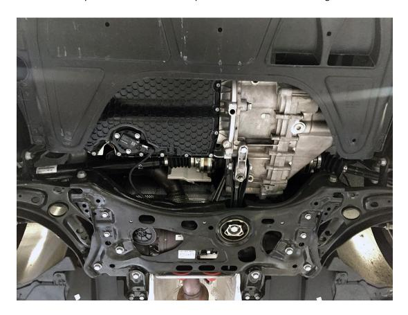
**Step 2** – Locate the factory dogbone mount, and notice the 21mm bolt securing the two halves to the factory torque arm, circled in red below.
