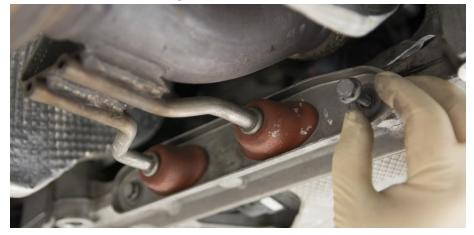
**Step 5** Using an 18mm Socket and extension, remove the front subframe bolts.
