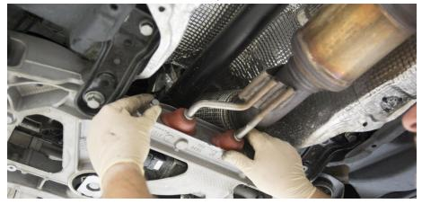
**Step 17** Verify that the subframe is properly aligned and all Locking Collars are fully seated. Torque the new Factory Subframe Bolts to **70 Nm + 180°.**
