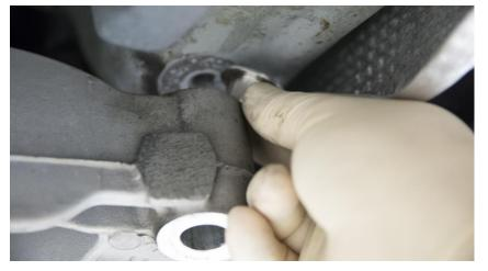
**Step 9** Install the two 601-0029 Locking Collars into the tops of the front subframe holes, as pictured below.
