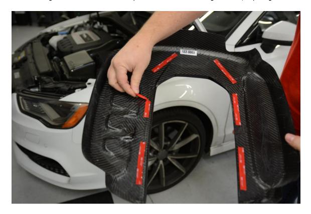
**Step 6** – Carefully begin setting the Carbon Fiber Engine Cover over the factory plastic part.
