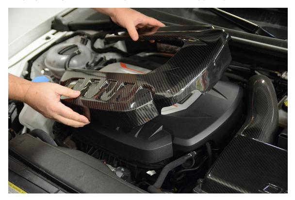
**Step 7** – Once the Carbon Fiber Engine Cover is properly aligned, press down firmly to ensure the adhesive strips stick to the plastic cover beneath it.
