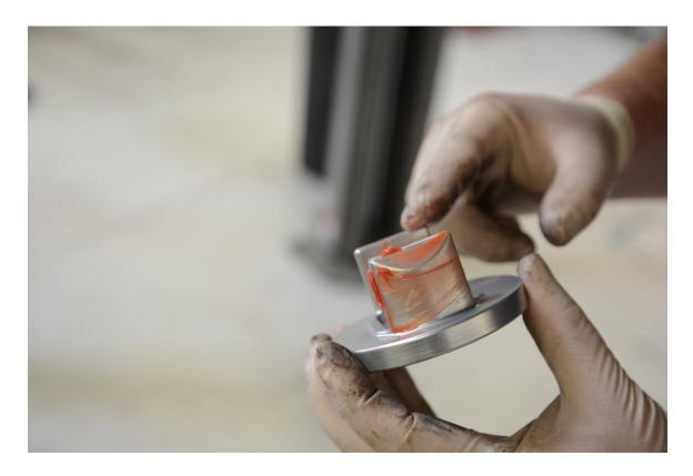
**Step 20** – Align the 034Motorsport Front Subframe Insert (601-0033) with the voids in the factory subframe bushing.
