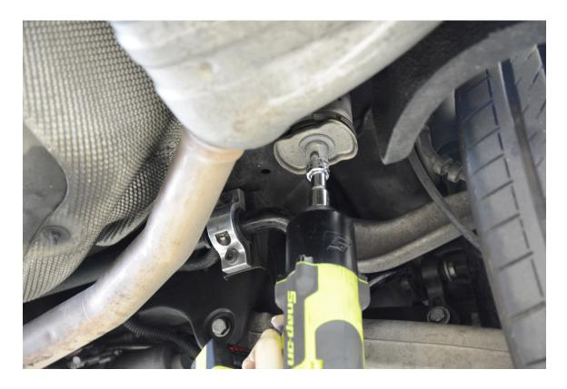
**Step 2** – Once the subframe bolt is removed, use a small pry bar to separate the factory washer from the rubber bushing.
