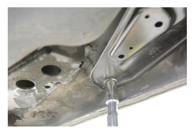
**Step 16** – Using an 18mm Socket (some vehicles will require a 21mm socket), remove the bolt securing the front of the rear subframe to the chassis, and remove the steel subframe mount bracket.
