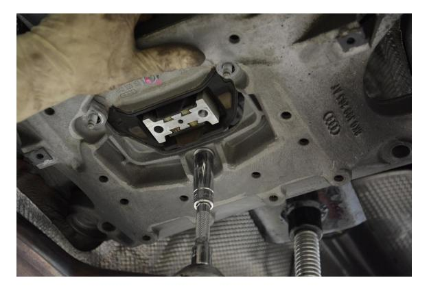
**Step 6** – Reinstall the factory transmission mount assembly carrier/crossmember to gain access to the factory transmission mount. Set this part aside as it will be reused later.
