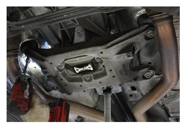
**Step 18** – Reinstall the securing the transmission mount limiter you removed in Step 3 and torque the two 10mm Triple Square bolts to 20 Nm. Better yet – replace it with a <u>034Motorsport B8/B8.5 Audi A4/S4/RS4, A5/S5/RS5, Q5/SQ5</u> <u>Transmission Mount Insert Upgrade</u>!
