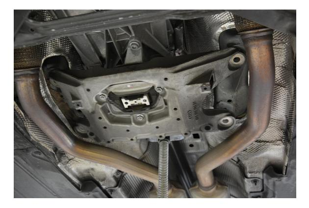
**Step 17** – Reinstall the four 12mm Triple Square bolts you removed in Step 4. Torque to 70 Nm. Torque the three 13mm Hex nuts you threaded on in Step 16 to 20 Nm.
