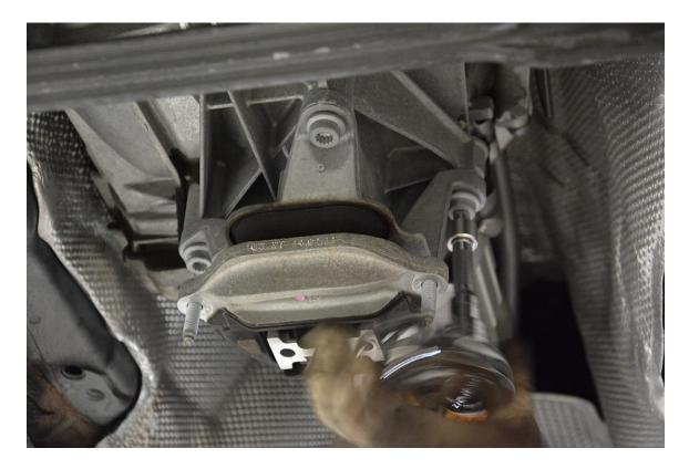
**Step 9** – Remove the 13mm Hex nut securing the transmission mount to the transmission mount bracket. Set this part aside as it will be reused later.
