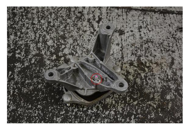
**Step 10** – Separate the transmission mount from the transmission mount bracket.
