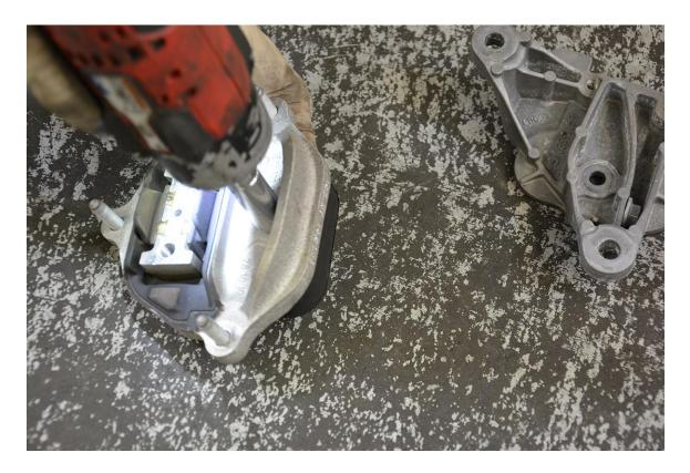
**Step 12** – Remove the factory rubber mount, and replace with the 034Motorsport Street Density Transmission Mount Upgrade.
