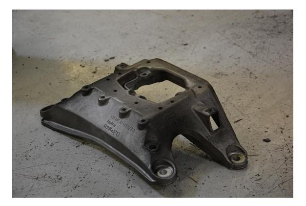
**Step 7** – Locate the factory transmission mount assembly, and remove the three 10mm Triple Square bolts securing it to the transmission. Set these parts aside as they will be reused later.
