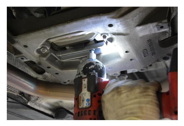
**Step 4** – Remove the four 12mm Triple Square bolts securing the transmission mount assembly carrier/crossmember to the chassis. Set these parts aside as they will be reused later. Only three nuts are now holding the crossmember in place, so be sure to support it or hold onto it before moving on to the next step.
