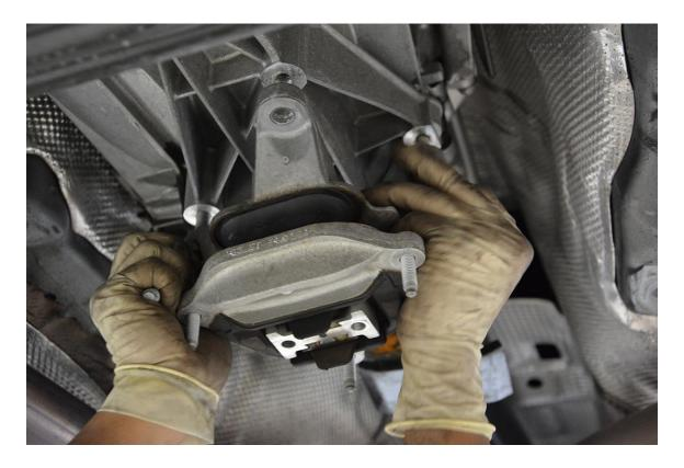
**Step 16** – Reinstall the crossmember you removed in Step 6 by loosely threading on the three 13mm Hex nuts you removed in Step 5.
