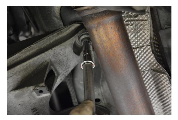
**Step 5** – While holding or supporting the crossmember, remove the final three 13mm Hex nuts securing it to the transmission mount assembly. Set these parts aside as they will be reused later.
