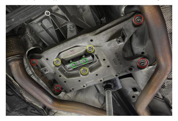
**Step 3** – Remove the two 10mm Triple Square bolts securing the transmission mount limiter. Set these parts aside as they will be reused later.
