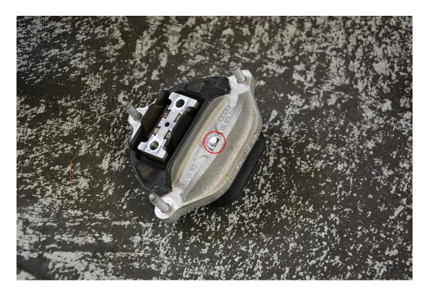
**Step 14** – Reinstall the transmission mount bracket you separated in Step 10 using the 13mm Hex nut you removed in Step 9. Please pay attention to the orientation of the bracket when reinstalling. Torque to 20 Nm.
