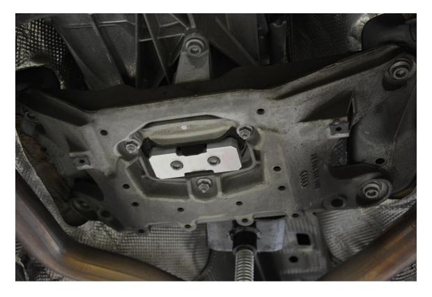
**Step 18** – Reinstall the undercarriage tray if you removed it, or just reinstall the two T25 Torx screws if you left it in place. You're all done! Enjoy further reduced drivetrain slop and improved launches, shifts, and throttle response!
