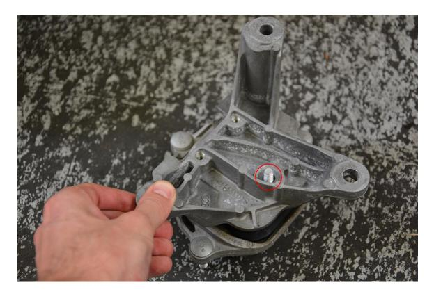
**Step 15** – Reinstall the transmission mount assembly using the three 10mm Triple Square bolts you removed in Step 7/8. Torque to 40 Nm.
