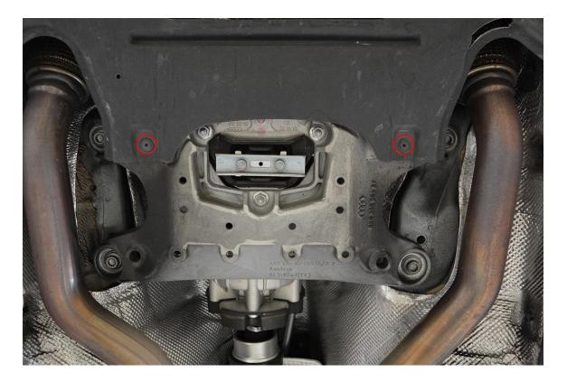
**Step 2** – Support the rear of the transmission using a screw type jack, as pictured below. You will be removing the fasteners circled below in the following order: Green (Q2 – 10mm Triple Square) >>> Red (Q4 - 12mm Triple Square) >>> Yellow (Q3 – 13mm Hex). **Important:** Support the transmission mount crossmember before removing the last 3 nuts.
