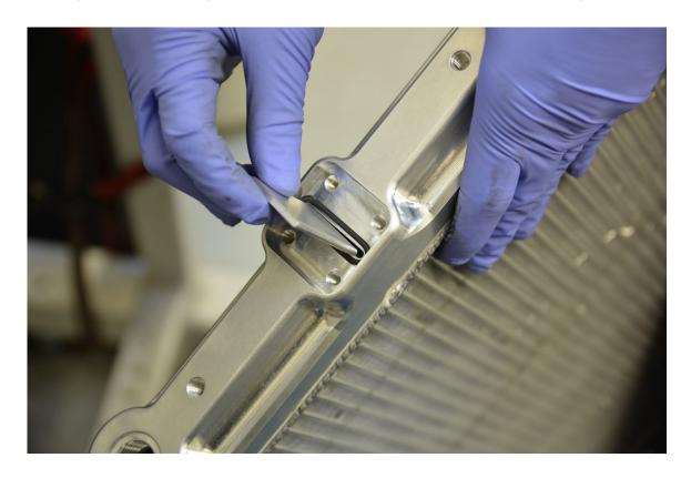
**Step 15b (B8.5 only)** –Diverter plate installed (driver side for RHD cars).
