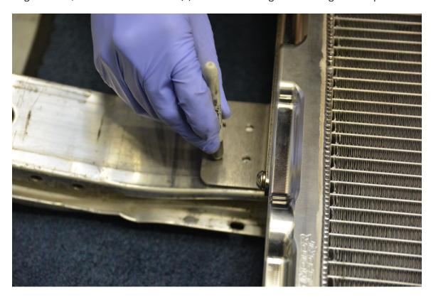
**Step 21 –** Using a center punch, mark center of each mark from step 20. This will make drilling much easier.
