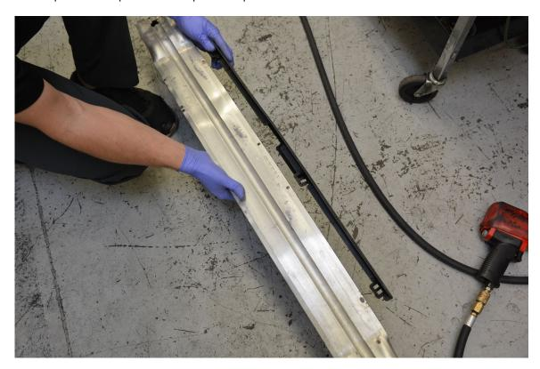
**Step14a -** Install 25x3 o-ring in groove in 034 heat exchanger end tanks.
