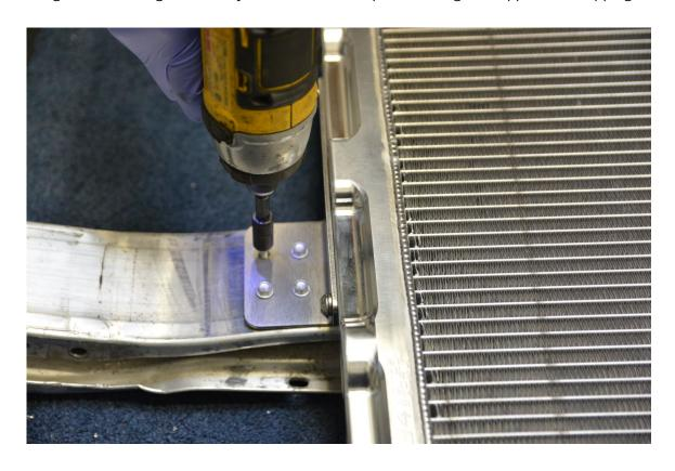
**Step 24 –** Drill 3/16" hole through bumper bar for zip-tie anchor.
