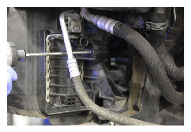
**Step 6** – Using a flat screw driver, disengage clip on right-hand end of factory heat exchanger.
