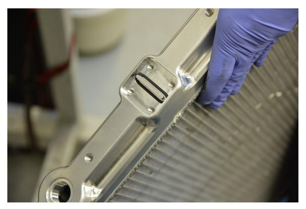
**Step 16** – Install cover plates. Use blue Loctite on M6x10 flat head screws. Hint: the top of the 034 heat exchanger is the side with threaded holes in the end of the end tanks for 1/8" NPT air bleed plugs.
