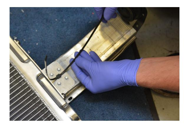
**Step 27 -** Assemble air block-off plates.
