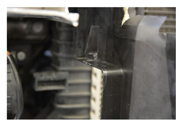
**Step 31 –** Remove backing from double sided tape and install air deflector plate, pressing firmly to attach tape.
