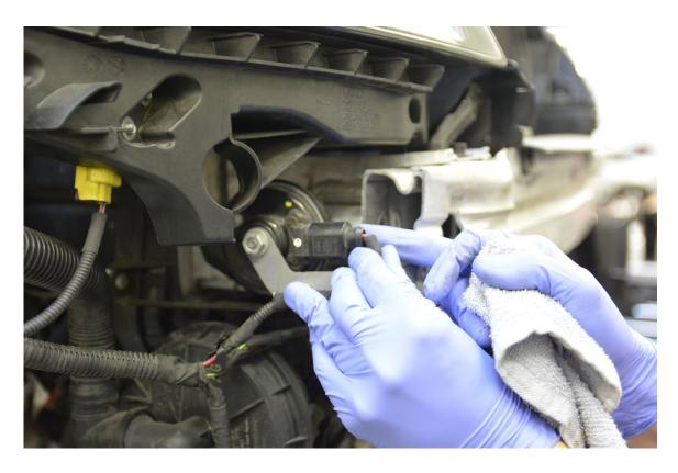
**Step 10** – Disconnect outside air temp sensor from plastic bracket. Be careful, bracket can be brittle.
