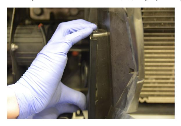
**Step 32 –** Install 90° fitting, hose and hose coupler.
