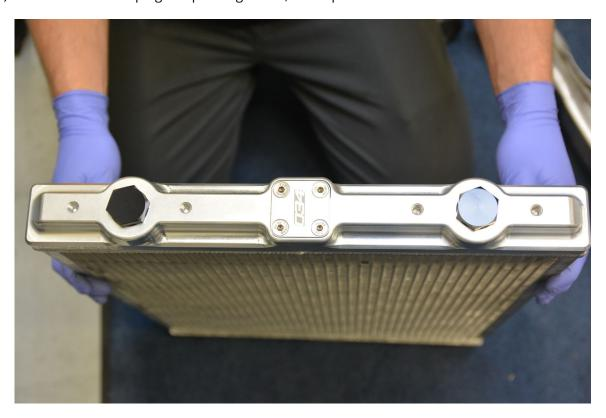
**Step 18 –** Install mounting brackets using M8x14 button head cap screws and M8 lock washer. Blue Loctite can also be added to screws. **Note:** bracket to bumper bar mounting flange points outward from heat exchanger.
