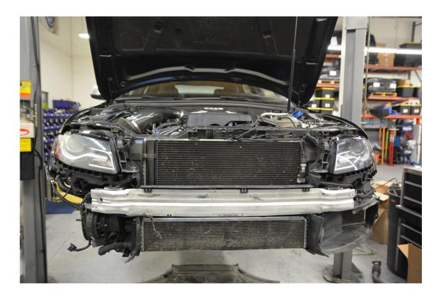
**Step 2** – Remove secondary radiator air duct.
