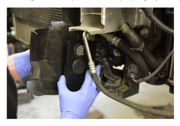
**Step 30 – (B8 only)** - Make a small notch in passenger side stock air deflector.
