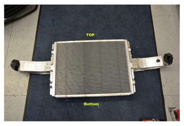
**Step 20 –** Using a marker, transfer locations of all (8) holes in mounting bracket flange to bumper bar.
