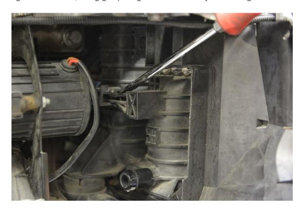
**Step 7** – Remove factory heat exchanger, careful not to damage factory plastic air ducts.
