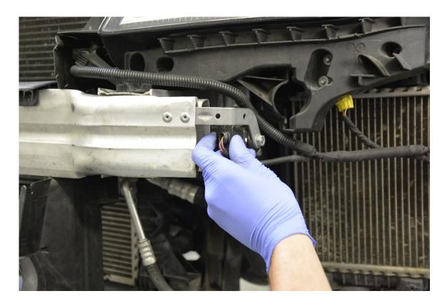
**Step 9** – Disconnect right side horn, and wire retaining clip.
