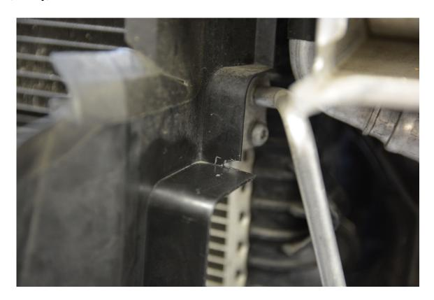
**Step 29 –** Remove backing from double sided tape and install air deflector plate, pressing firmly to attach tape.
