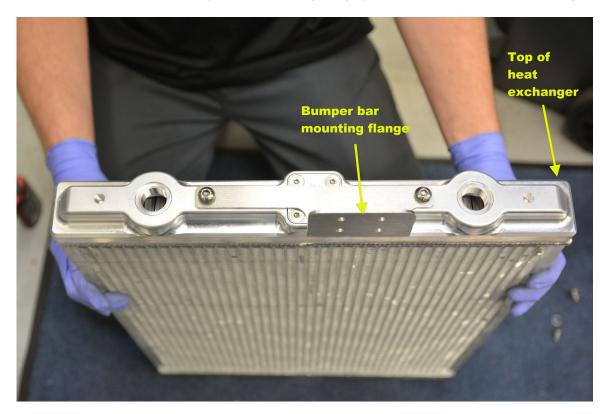
**Step 19** -With bumper bar facing downward, place heat exchanger assembly on it, centered.
