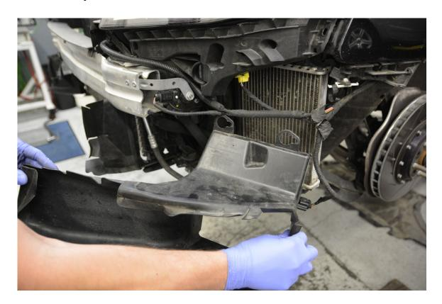
**Step 3** – Placing a suitable catch pan underneath, remove lower heat exchanger hose using pliers, or spring clamp pliers.
