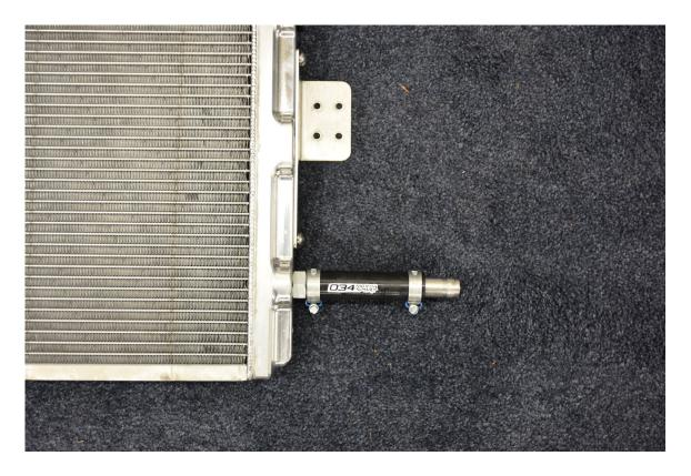
**Step 34 –** Install heat exchanger assembly. Run silicone hoses through grommets in air deflector plates, and connect to stock lines.
