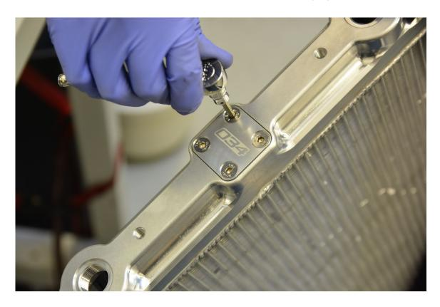
**Step 17 –** Install -10AN plugs. **NOTE:** B8 will have a plug on each end; top on passenger side, bottom on driver side (RHD cars). B8.5 will have both plugs on passenger side, like in photo.
