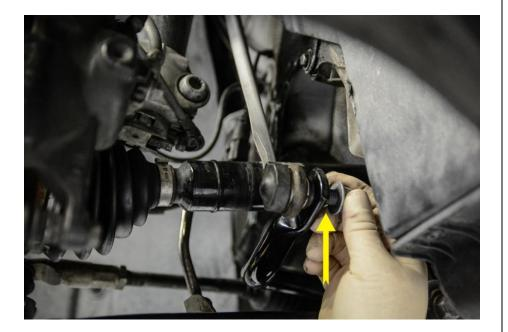
**Hint:** The outer hole is the "Soft" setting, and the inner hole is the "Stiff" setting.
