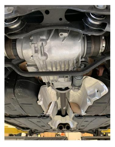
**Step 10**Remove the press-nuts from the underbody heat shielding.
