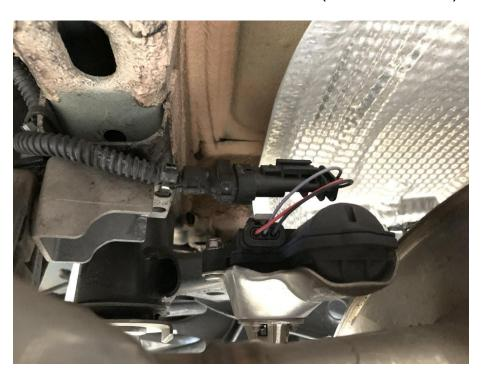
**Step 8**Remove the 3 exhaust hanger bracket bolts.
