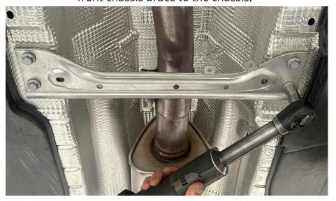
**Step 10**Remove the front chassis brace.
