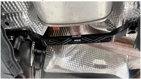
**Step 7**Torque the hardware to **20Nm.**
