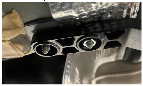
**Step 7**Torque the hardware to **20Nm.**
