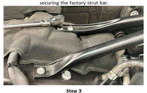
Using a 10mm socket, remove the nuts from the firewall brackets.
