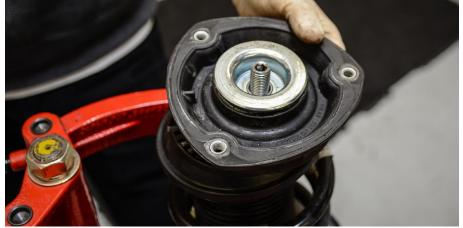
**Step 14** The window to access the upper strut nut will lean towards the windshield once installed.
