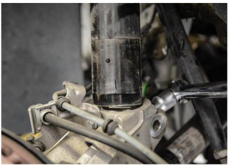
Use a 13mm Socket to remove the strut mount bolts.
