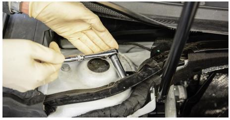
**Step 5** With the dust shield out of the way, you'll notice the easy access to the 3 strut mount bolts for later.
