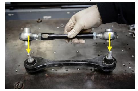
Align the bolt holes of 034Motorsport Density Line Adjustable Rear Toe Link with the rear hub assembly.
