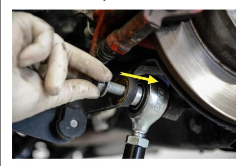
Position the inner rod end within the rear subframe provisions and align bolt holes.
