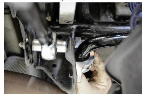
Double check the installation and verify that all sway bar connections are torqued to spec. Either use pole jacks to lift the rear suspension or use an alignment rack or service pit to torque the inner and outer toe link bolts on both sides
