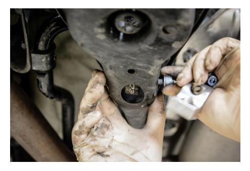
Locate the 2 bolts (inner and outer) securing the factory rear toe link to the rear subframe and rear hub assembly
