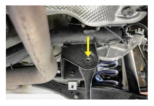
Set the new 034Motorsport Density Line Adjustable Rear Toe Link to the same length as the factory toe link by aligning the bolts through both the factory and 034Motorsport rear toe links simultaneously
