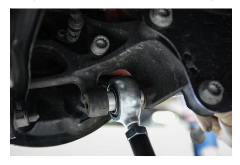
\*Position such that the short spacers are on the outside (hub assembly) and taller spacers mount to the rear subframe
