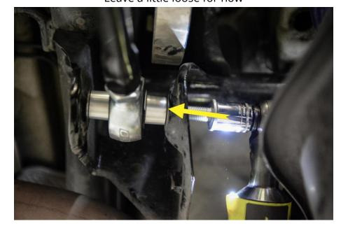
Reinstall the lower rear sway bar end link bolt, securing the rear sway bar end link to the lower rear control arm. Torque to **35 Nm**.
