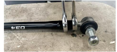
Use (2x) 19mm wrenches to lock the jam nuts at the desired length. (Dynamic+ links shown, tighten while on the car)
