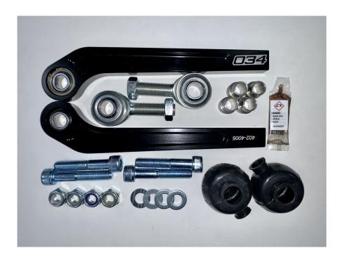
**Step B**Apply half packet of anti-seize to spherical heim joint
