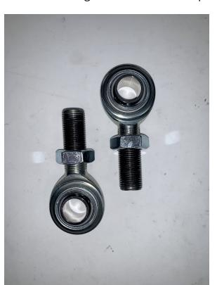
Install the heim joint into the billet end links, leaving about 2-3 threads exposed
