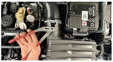
**Step 6**Separate the intake hose from the airbox.
