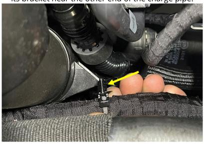
**Step 16**Pull charge pipe away the from lower intake hose.
