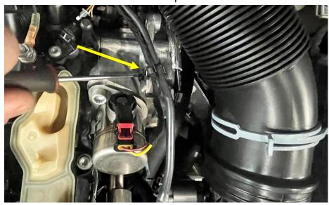
**Step 8**Disconnect cam position sensor.
