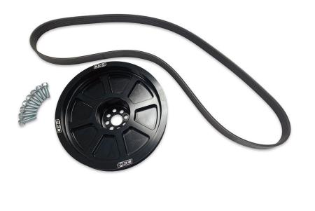
034Motorsport's Lower Supercharger Pulley is the new standard in performance and durability. This pulley was engineered with performance, light weight, and discrete good looks, in mind. Manufactured from billet 6061-T6 aluminum, for strength and long lasting reliability.
