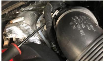
**Step 4** Squeeze the tabs on the turbo recirculation adapter to release it from the airbox.
