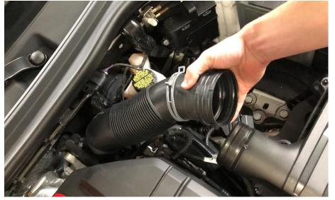
**Step 6** Install the 034 intake hose into the stock location.
