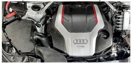
**Step 2**Remove the engine cover by pulling upward.
