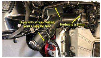
**Step 7** Unclip the secondary air injection hose by squeezing the tabs and pulling downwards.
