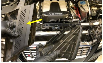
**Step 5** Remove the Rear Engine cover and set aside gently.
