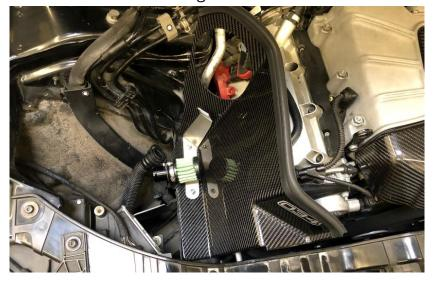
**Step 13** Install the secondary air hose to the adapter.
