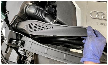
**Step 6**Remove the engine cover by pulling upward.
