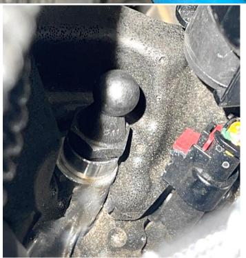
**Step 14** Install the 034 ignition coils.
