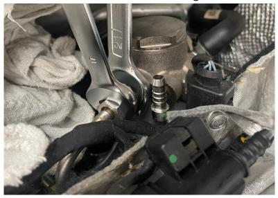
**Step 34**Reinstall the pressure sensor connector.
