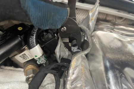
**Step 36**Button up the heat jacket for the fuel lines.
