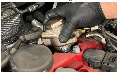
Step 26 Using a 10mm triple square bit, reinstall the HPFP. Torque to 20Nm.
