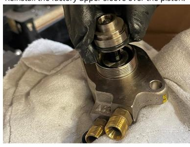
**Step 21**Reinstall the retaining nut to the HPFP assembly.
