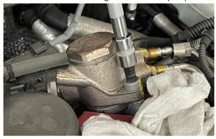
**Step 12**Remove the electrical connector from the HPFP.
