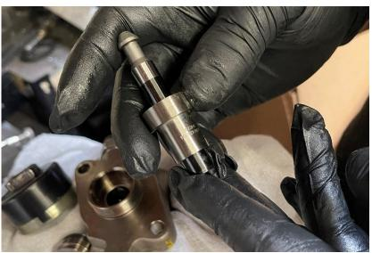
**Step 20**Reinstall the factory upper sleeve over the piston.
