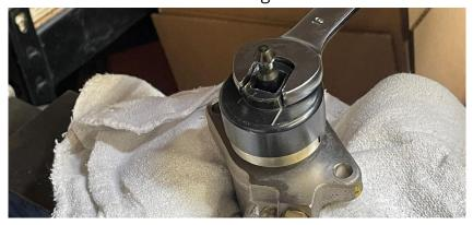
**Step 17** Extract the piston and upper sleeve from the fuel pump.
