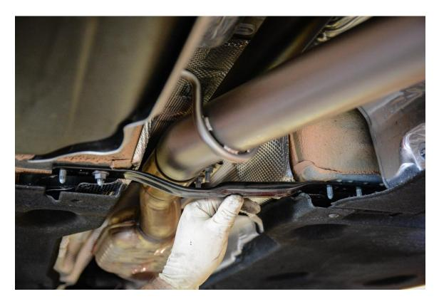
**Step 19 –** Check that exhaust clamps are secure. Lower vehicle from jackstands or lift, and enjoy the new roar of your 2.0T Gen 3!
