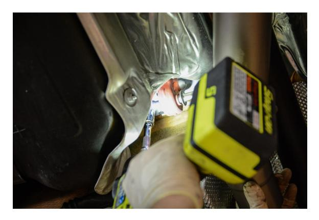
**Step 16 –** Ensure the clamp is covering equal amounts of the factory downpipe and 034Motorsport Res-X Resonator Delete. Using a 13mm Socket, tighten the 2 nuts on the factory exhaust clamp.
