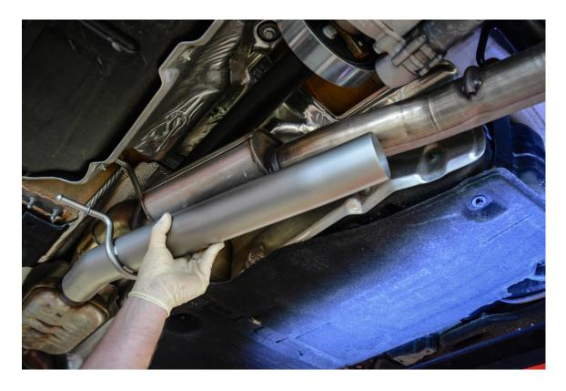
**Step 4** – This mark will be where you cut the factory resonator from the rear exhaust portion.
