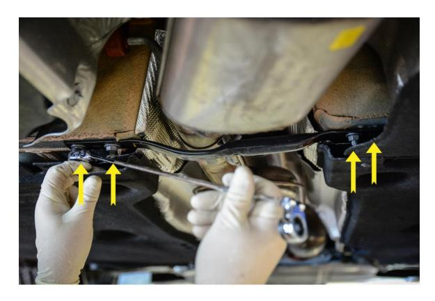
**Step 3** – Line up the 034Motorsport Res-X Resonator Delete underneath the factory resonator. Once aligned, mark the end of the 034Motorsport Res-X Resonator Delete on the factory exhaust with a pen.
