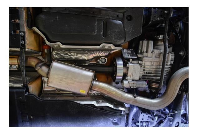
**Step 2** – Using a 13mm Wrench or Socket, remove the 4 nuts securing the factory brace to the chassis below the exhaust tunnel.
