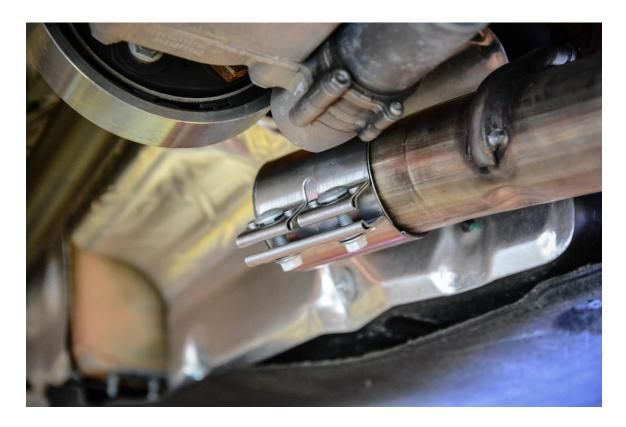
**Step 14 –** Slide the factory exhaust clamp onto factory downpipe loosely. Then slide 034Motorsport Res-X Resonator Delete into rear section of the factory exhaust. Ensure the clamp is covering equal amounts of factory exhaust and 034Motorsport Res-X Resonator Delete.
