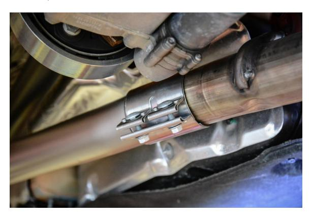
**Step 15 –** Using a 13mm Socket, install the bolt securing the exhaust hanger bracket to the chassis. Torque to **20 Nm.**
