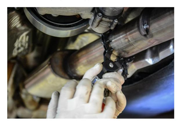
**Step 8** – Using a 13mm Socket, loosen the 2 nuts on the factory exhaust butt clamp before the resonator.
