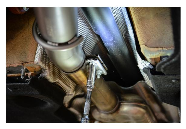
**Step 17 –** Using a 15mm Socket, tighten the 2 nuts on the exhaust clamp securing the rear portion of the 034Motorsport Res-X Resonator Delete to the factory exhaust.
