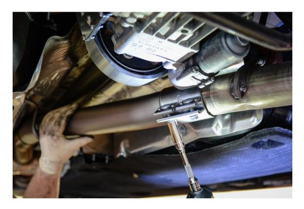
**Step 18** –Reinstall the factory tunnel brace and install the 4 nuts securing brace to chassis with a 13mm Socket. Torque nuts to **20 Nm.**
