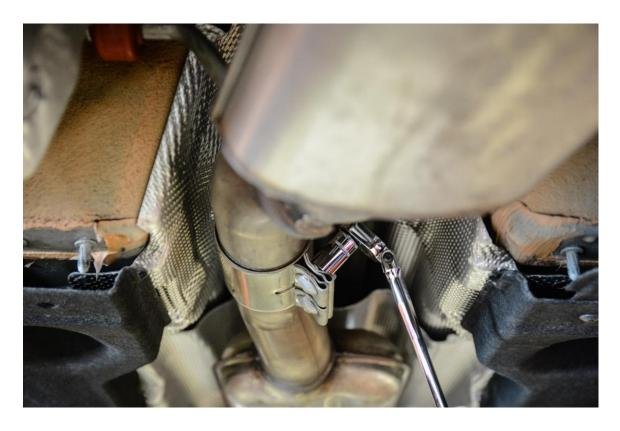
**Step 9** – Using a 13mm Socket, remove the bolt securing the factory exhaust hanger to the chassis. The resonator should now be free and removed from the car.
