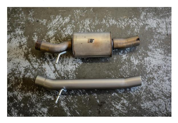
**Step 12 –** Install the factory exhaust hanger and bracket to the 034Motorsport Res-X Resonator Delete.
