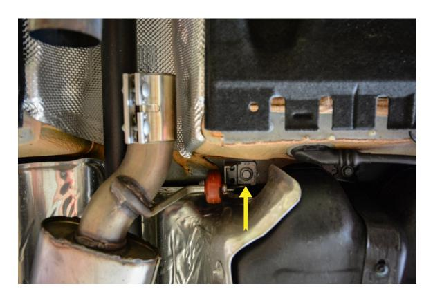
**Step 10** – Remove the factory rubber exhaust hanger and bracket from the factory resonator.
