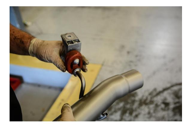
**Step 13 –** Loosely pre-install the supplied exhaust butt clamp on the rear portion of the factory exhaust.
