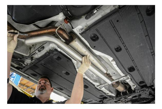
**Step 4** – This mark will be where you cut the factory resonator from the rear exhaust portion.
