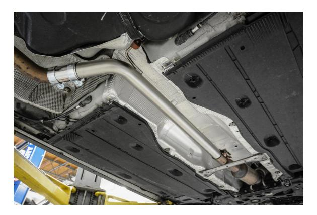
**Step 14 –** Using a 12mm socket, tighten the 2 nuts of the exhaust clamp securing the rear portion of the factory exhaust to the rear of the Res-X Resonator Delete.
