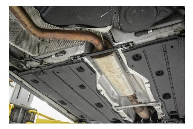
**Step 2** – Using a 13mm socket, remove the 4 nuts securing the factory brace to the chassis below the exhaust tunnel.
