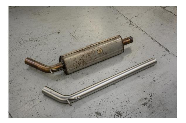
**Step 11** – With the supplied butt clamp loosely installed, align the rear portion of the Res-X Resonator Delete with the factory exhaust. Be sure to install the welded support into the factory rubber hanger.
