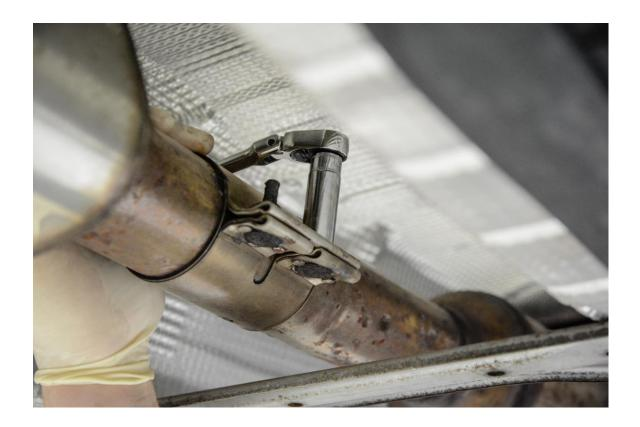
**Step 9** – Using a pair of pliers, carefully remove the factory resonator from the rubber hanger and lower out of the car.
