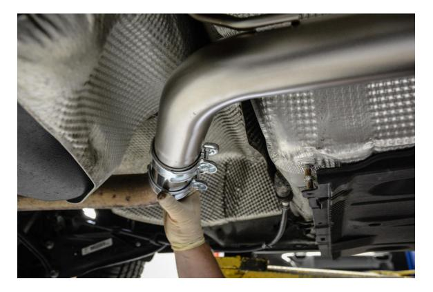
**Step 12** – Now align the front of the Res-X Resonator Delete with the factory downpipe. Loosely slip the factory butt clamp over the seam, so that it evenly covers the Res-X and downpipe.
