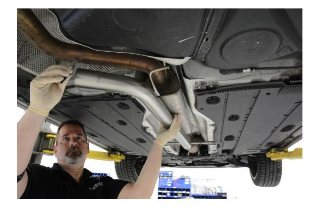
**Step 5** – We found the best way to cut the factory exhaust behind the resonator was using a pipe cutter. These can be found at most hardware stores.
