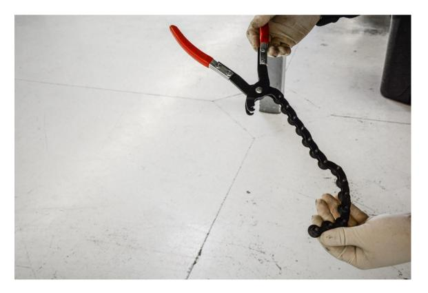
**Step 6** –Line up the pipe cutter over the factory exhaust along the line you just made. **Tip:** Double check that you're cutting the pipe as straight as possible for proper alignment.
