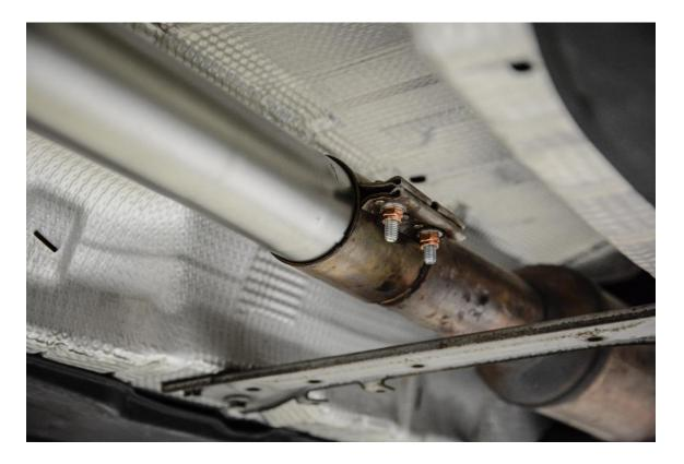
**Step 16 –** Using a 13mm socket, reinstall the tunnel brace and 4 factory nuts to the chassis.
