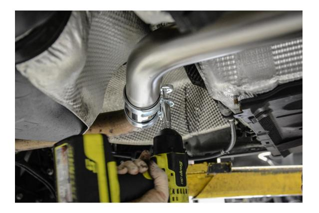
**Step 15** – Using a 13mm socket, tighten the 2 nuts of the factory exhaust clamp, securing the downpipe to the front of the Res-X Resonator Delete.
