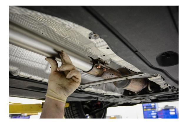
**Step 13** – Check the alignment of the Res-X Resonator Delete relative to the factory exhaust components while the clamps are loose. Adjust as necessary.
