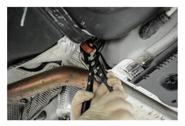
**Step 10** – The factory resonator should now be completely free from the underside of the car. Here's a comparison of the large factory resonator to the compact, 034Motorsport Res-X Resonator Delete.
