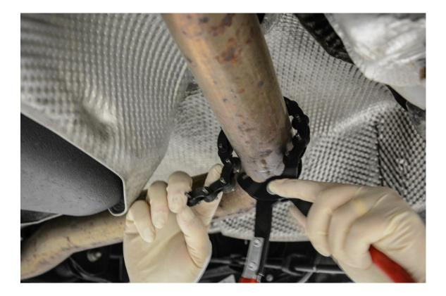
**Step 7** – Check that you've cut completely around the pipe.
