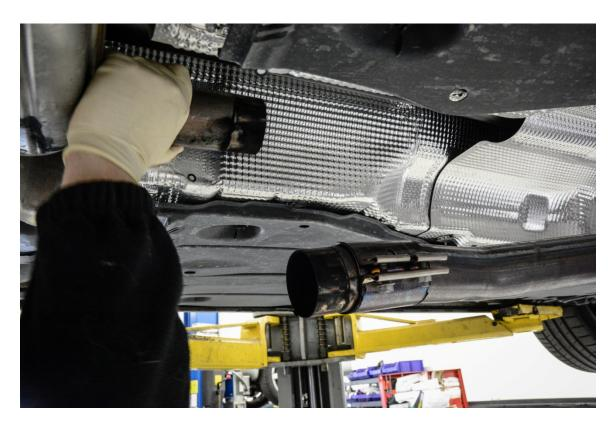
**Step 11** – Ensure that the cut made to the factory exhaust behind the resonator is complete. If so, the resonator should now be free and removed from the car. Keep the existing factory exhaust clamp on the downpipe.
