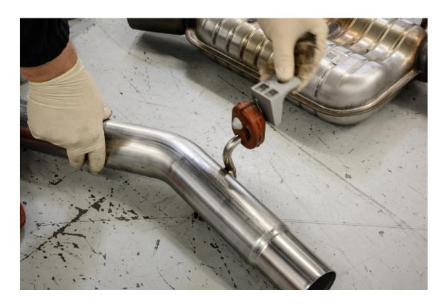
**Step 14 –** Slide 034Motorsport Res-X Resonator Delete into front section of the factory exhaust. Ensure the clamp is covering equal amounts of factory exhaust and 034Motorsport Res-X Resonator Delete.
