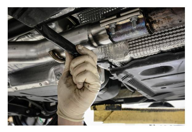
**Step 20 –** Check that exhaust clamps are secure. Lower vehicle from the jackstands or lift, and enjoy the new roar of your 2.0T Gen 3!
