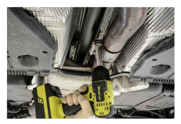
**Step 8** – Using a 13mm Socket, remove the bolt securing the exhaust hanger to the chassis.
