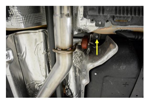
**Step 17 –** Using a 13mm Socket, tighten the 2 nuts on the OE exhaust clamp securing the front portion of the 034Motorsport Res-X Resonator Delete to the factory exhaust.
