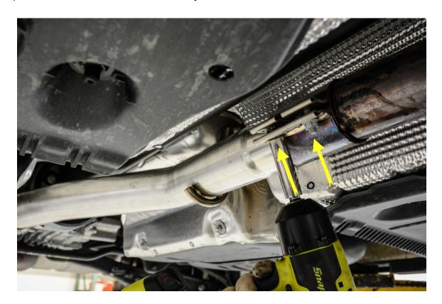
**Step 18 – Tip:** Rotate the rear exhaust clamp to leave clearance for the rear differential. Once in place, use a 13mm Socket to tighten the 2 nuts securing the exhaust clamp to the 034Motorsport Res-X Resonator Delete and rear portion of exhaust.
