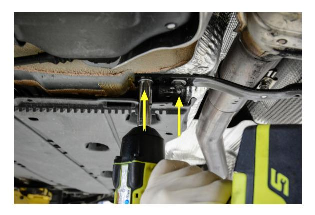
**Step 10** – Slide the factory exhaust butt clamp forward and out of the way. The front of the resonator should now be free from the downpipe.
