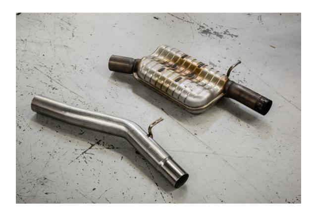
**Step 13** – Remove the factory exhaust hanger and bracket from the resonator, and transfer to 034Motorsport Res-X Resonator Delete. Preinstall the supplied exhaust clamp on rear portion of the 034Motorsport Res-X Resonator Delete.
